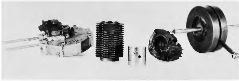
FIGURE 12.—De Dion-Bouton engine. Left to right: crankcase section (ignition side), cylinder, piston, cylinder head, crankshaft with connecting rod and flywheel unit. (Smithsonian photo A4474.)
