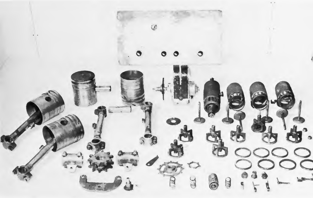
Figure 7.—First flight engine, 1903: cylinder, valve box, and gear mechanism; below, miscellaneous parts. (Photos courtesy Science Museum, London, and Louis P. Christman.)
