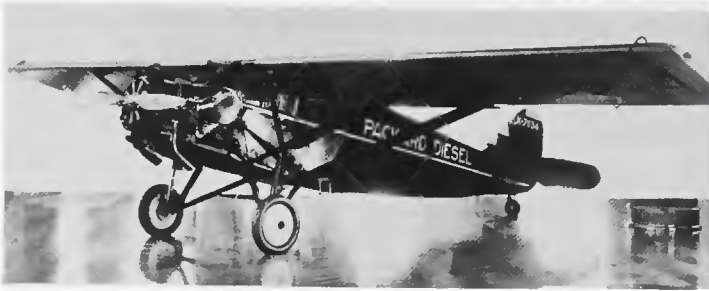
Figure 6.—Stinson SM-1DX "Detroit." This airplane, powered with original Packard DR-980 diesel engine, made the world's first diesel-powered flight on September 19, 1928. (Photo courtesy of Henry Ford Museum, Dearborn, Michigan.)
