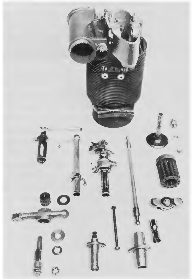
Figure 28.—Cylinder disassembly, showing valve and fuel injector. U.S. Navy test, 1931. (Smithsonian photo A48324D.)
