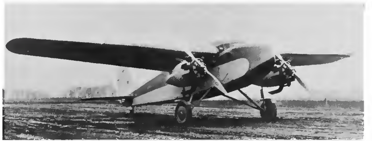
Figure 12.—Stewart M-2 Monoplane, 1930, with 2 Packard 225-hp DR-980 diesel engines. (Smithsonian photo A48319C.)
