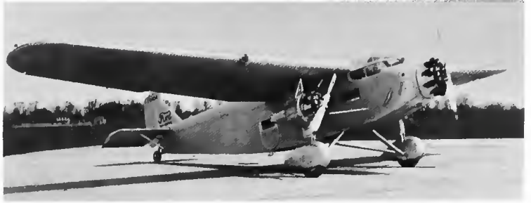
Figure 10.—Ford 11-AT-1 Trimotor, 1930, with 3 Packard 225-hp DR-980 diesel engines. Note special bracing for the outboard nacelles. (Smithsonian photo A48311B.)
