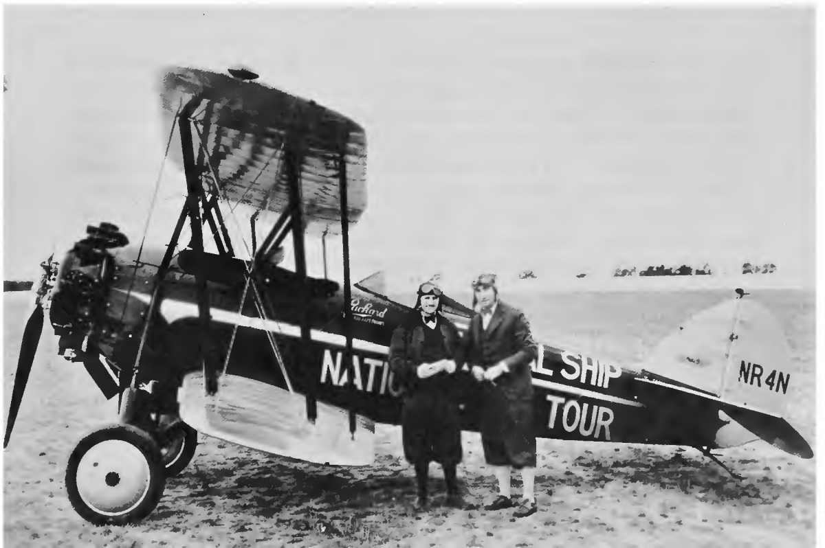
Figure 15.—Walter E. Lees, official timer, and Ray Collins, manager, 1930 National Air Tour, with their official airplane, a Packard diesel Waco "Taper Wing," at Packard proving grounds near Detroit. (Smithsonian photo A49449.)
