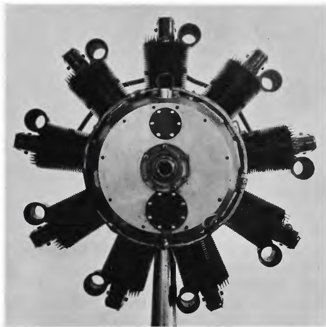
Figure 1 (left).— Front view of first Packard diesel, 1928. Note hoop holding cylinders in place and absence of venturi throttles. This engine was equipped with an air pressure starting system. (Smithsonian photo A2388.) Figure 2 (right).— Left side view of first Packard diesel, 1928. Heywood starter (air) fitting shown on the head of the next to lowest cylinder. (Smithsonian photo A2388C.)
