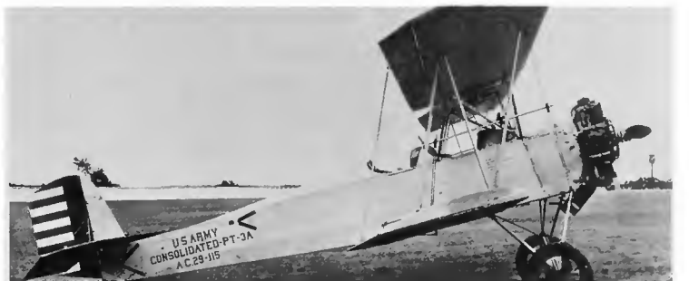
Figure 13.—Consolidated XPT-8A, 1930. This is a Consolidated PT-3A powered by a DR-980 Packard diesel. (Smithsonian photo A48319E.)
