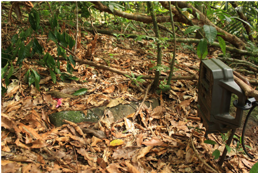
Fig. 2 Motion-sensitive camera trap mounted on a U-shaped concrete-reinforcement bar, used to monitor removal of seeds from an experimental station or from a cache
