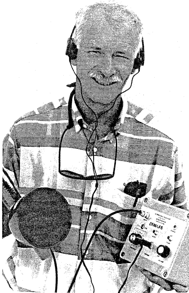
Figure 1. Commercial (Sonotronics) ultrasonic receiver with headphones and directional hydrophone.
