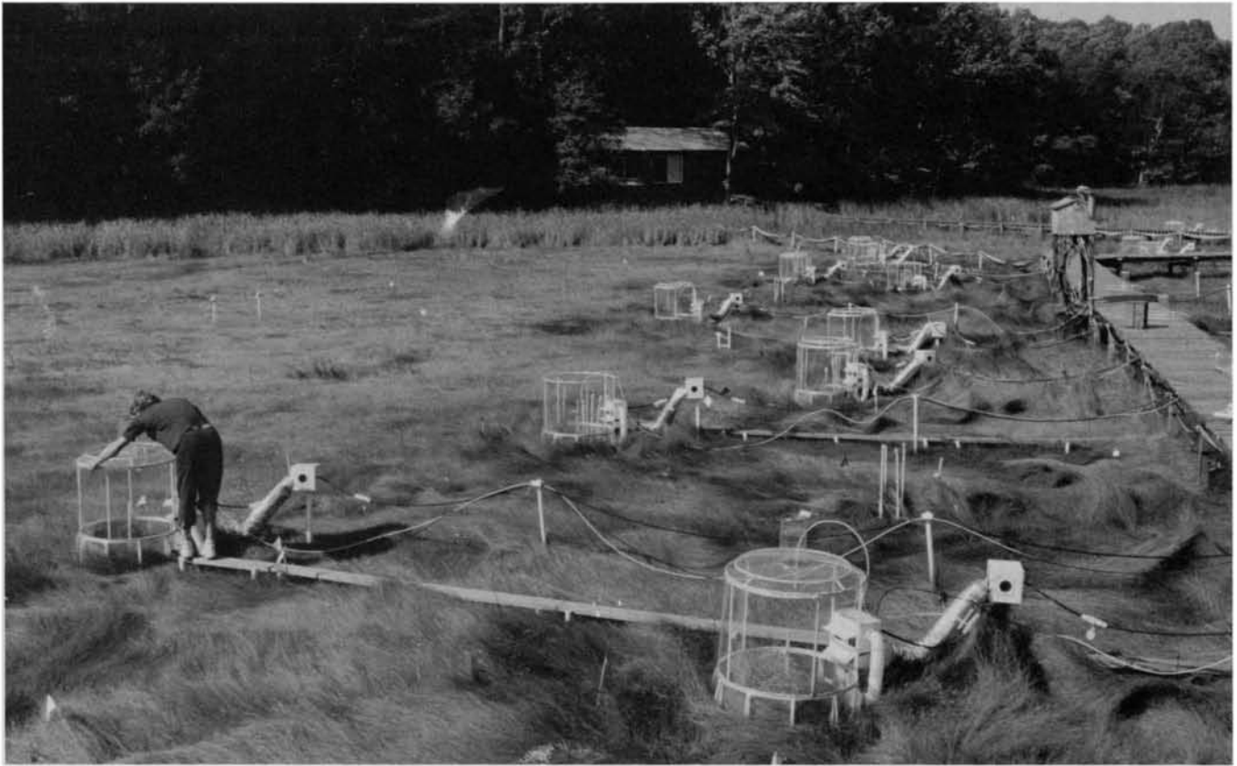
Figure 2. Open-top CO 2 -controlled chamber system used in the salt marsh on the Chesapeake Bay.
