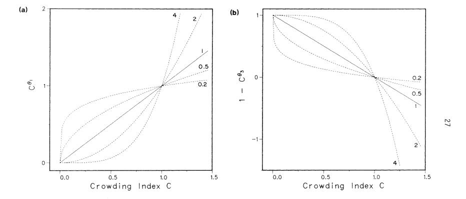
Figure 2.1. Power functions of the crowding index. (a) plots the function  $M_r = C^{\theta\,l}$  against C for the indicated values of  $\theta_l$  while (b) plots  $G_r = 1 - C^{\theta\,3}$ . The powers  $\theta_l$  and  $\theta_3$  adjust how suddenly each function changes near the critical value C = 1.
