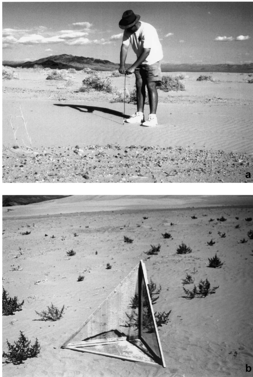
Fig. 7. (a) Technique for measuring sand thickness. Bare gravel surface in the foreground with 5–10-cm-thick sand being measured. (b) Corner reflector used to aid in registering radar images. The hypotenuse of each side triangle is \sim 1.4 m.
