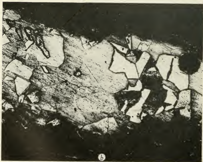
Photomicrographs of native copper. a , Microstructure of cross section of bead ( \times 100 ). b , Microstructure of cross section of amorphous fragment ( \times 100 ).
