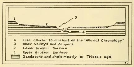
FIGURE 33.—Generalized section to show the relation of the two erosion surfaces, the inner canyons, and the alluvial formations.
