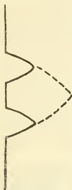
FIGURE 3.—Manner of cutting tree preparatory to felling.
