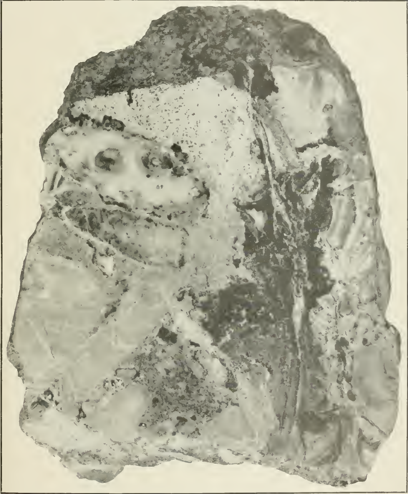
REPLACEMENT OF LIMESTONE CONGLOMERATE ALONG FISSURE
