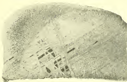
1. THE SIGNAL MOUNTAIN, LOWER CALIFORNIA, OCTAHEDRITE. MAGNIFIED 2\frac{1}{2} DIAMETERS: SHOWING IN THE UPPER LEFT SECONDARY GRANULATION.
