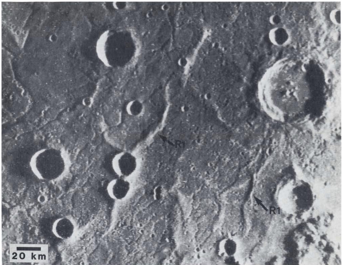
Fig. 7. Ridges in the Caloris Basin of Mercury. First-order ridges ( R_1 ) and arches are the only members of the ridge assemblage that have been observed. Second- and third-order ridges may exist but cannot be resolved in Mariner 10 imagery (Mariner 10, FDS 126).
