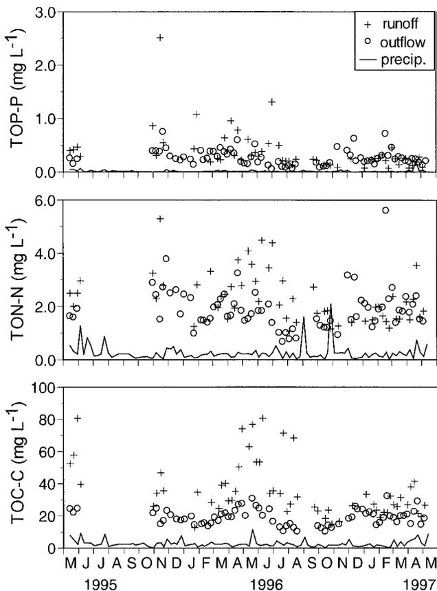
Fig. 6. Concentrations of total organic nitrogen (TON), phosphorus (TOP), and carbon (TOC) in inflowing runoff (+), out flowing water (o), and precipitation (line) in mg L<sup>-1</sup> N, P, or C.
