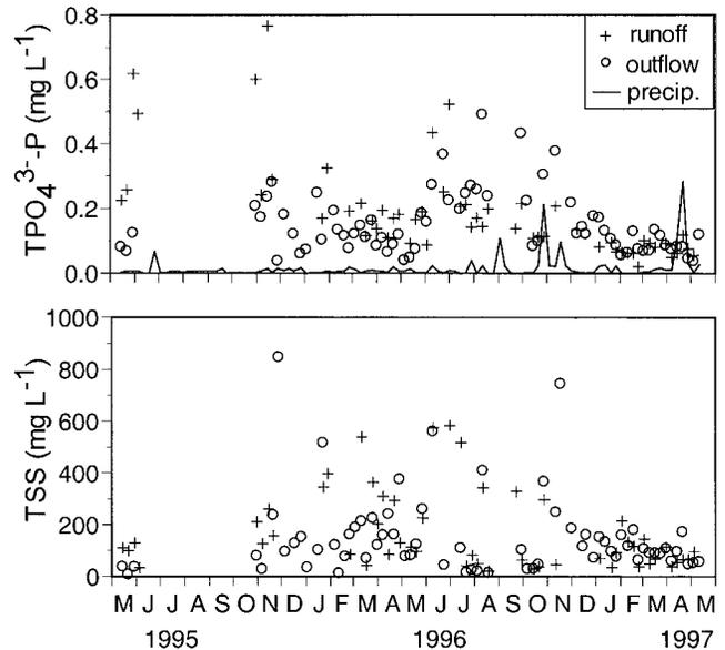
Fig. 7. Concentrations of total phosphate (TPO<sub>4</sub><sup>3-</sup>) and total suspended solids (TSS) in inflowing runoff (+), out flowing water (o), and precipitation (line) in mg L<sup>-1</sup> P or TSS.
