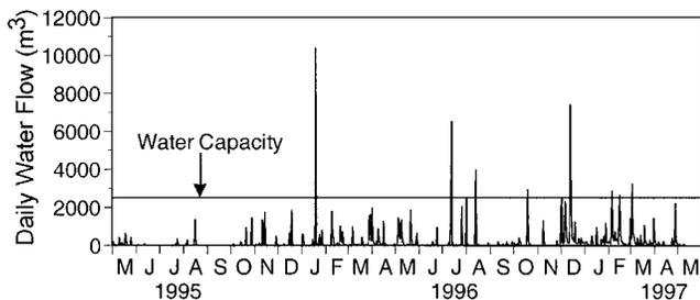
**Fig. 4.** Daily outflow of water vs. time for the wetland. The horizontal line at  $2500 \text{ m}^3$  indicates the water capacity (i.e., the volume held by the wetland before outflow occurs).
