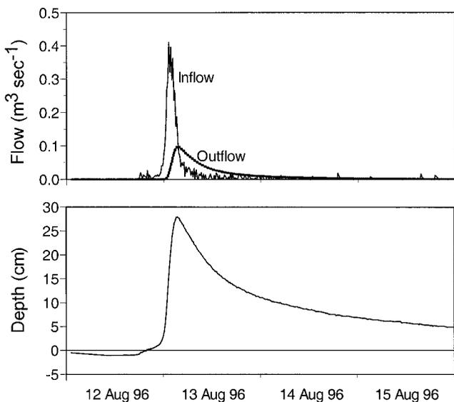
**Fig. 3.** Total inflow (from runoff and direct precipitation combined) and outflow of water and depth relative to bottom of V-notch in weir during a four-day period in August 1996. A rainfall and runoff event began late on 12 August.
