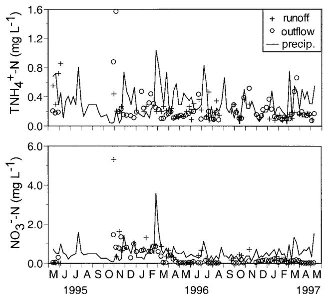
Fig. 8. Concentrations of total ammonium (TNH<sub>4</sub><sup>+</sup>) and nitrate plus nitrite (NO<sub>3</sub><sup>-</sup>) in inflowing runoff (+), out flowing water (o), and precipitation (line) in mg L<sup>-1</sup> N.
