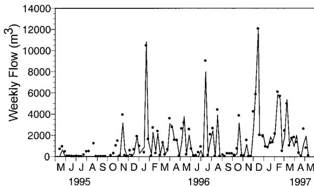
**Fig. 5.** Total inflow (points) and outflow (line) of water vs. time during the sampling intervals, which are approximately one week long.
