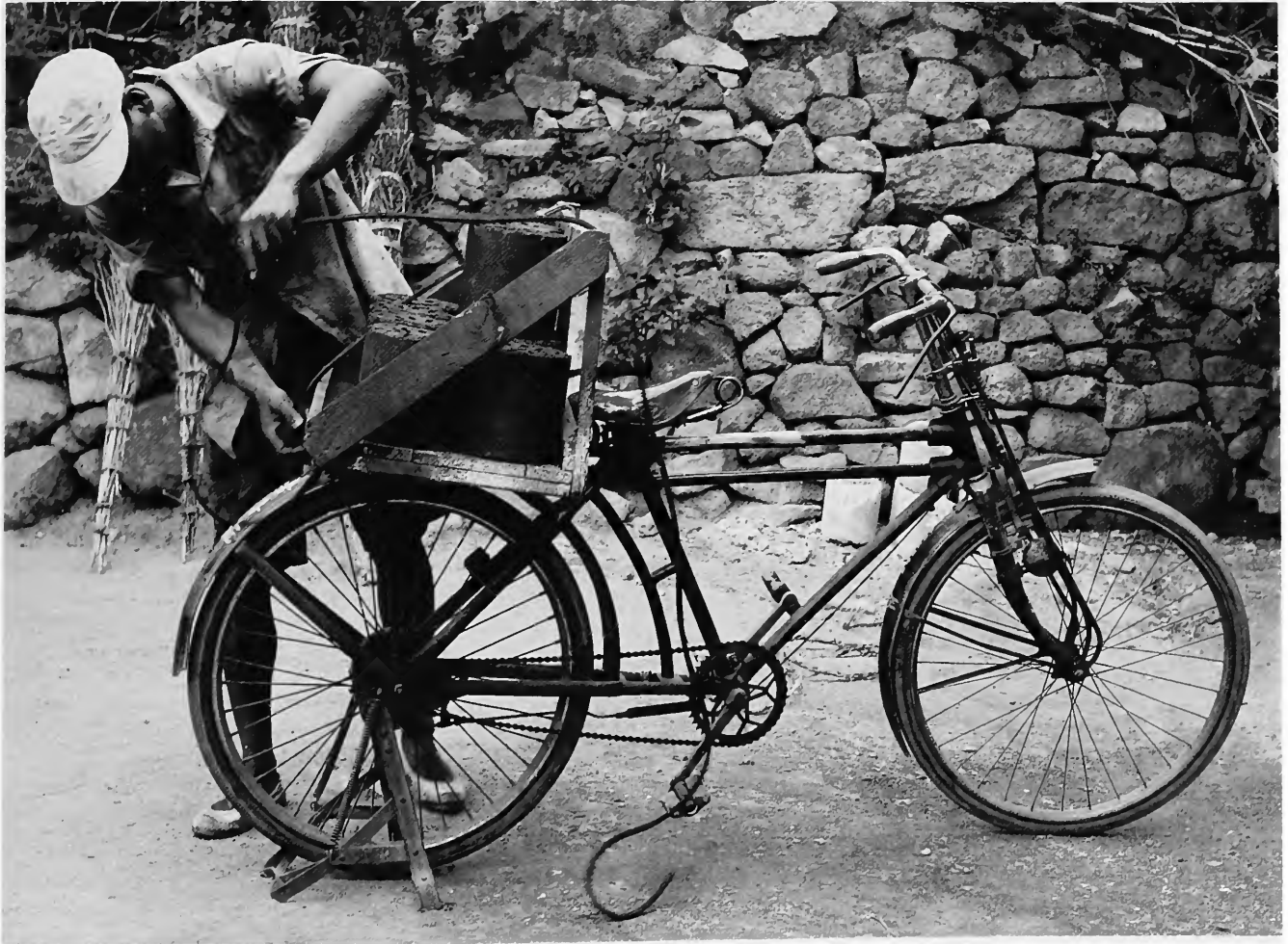
FIGURE 177.—Steel bicycle with an iron rack and stand for heavy-duty use. Black and white photograph, 1971.
