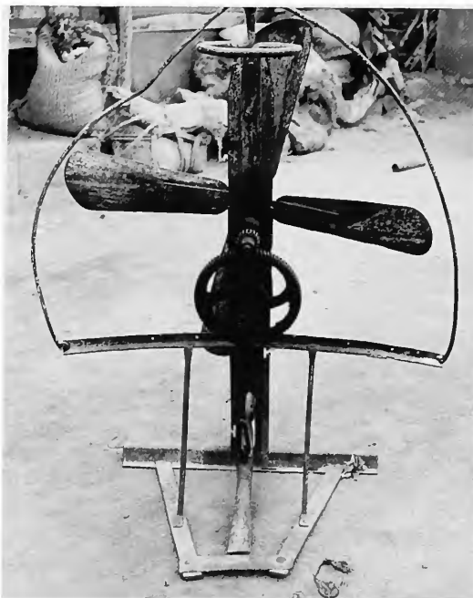
FIGURE 127.—Mechanical winnowing fan made of iron. Black and white photograph, 1955.
