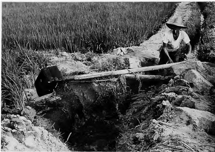
FIGURE 136.—Water-lift, operated as a lever with a scoop at one end to transfer irrigation water. Black and white photograph, 1960.
