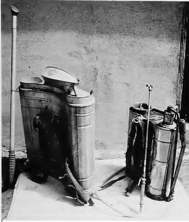
FIGURE 130.—Sprayers for fertilizer and insecticide, with pump handles and shoulder straps. From a color photograph, 1970.
