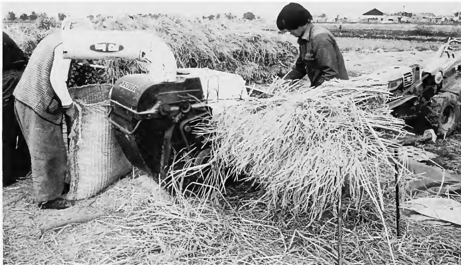
FIGURE 42.—A rotary thresher is powered by a belt attachment to a nearby motorized cultivator. From a color photograph, 1971.
