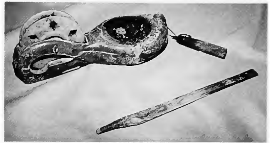
FIGURE 169.—Japanese carpenter's snap-line marker (pine) and a bamboo stylus. Black and white photograph, 1969.
