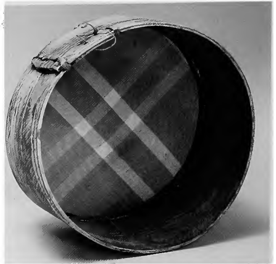
FIGURE 141.—Horsehair sieve, sometimes made from wisteria vine, more recently made with a screen of metal or plastic and having a stitched willow rim. Black and white photograph, 1955.
