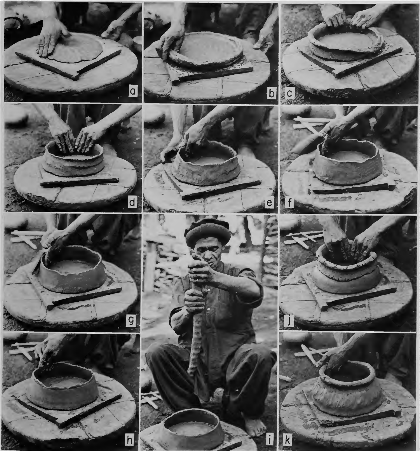
PLATE 3.—Stages in forming a water jar, Bomboret Valley, NWFP: a , flattening clay for base of vessel on turntable; b , raising edges; c , thinning lower wall by pinching; d , e , refining and smoothing lower wall; f , g , further thinning lower wall with beater (note that no anvil is used); h , trimming top ledge of lower wall; i , forming coil; j , k , bonding coil to top ledge of lower wall of vessel.
