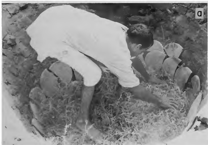
PLATE 36.—Setting a kiln, Garhi Maqbulabad, Gujrat (continued): a , placing a layer of straw over the sherds; b , placing a layer of flat dung pieces on the straw; c , a layer of coarse lumps of dung placed next; d , setting of a layer of tobacco bowls (note plank placed across top of kiln so potter can easily reach center of setting). (See Plate 37.)
