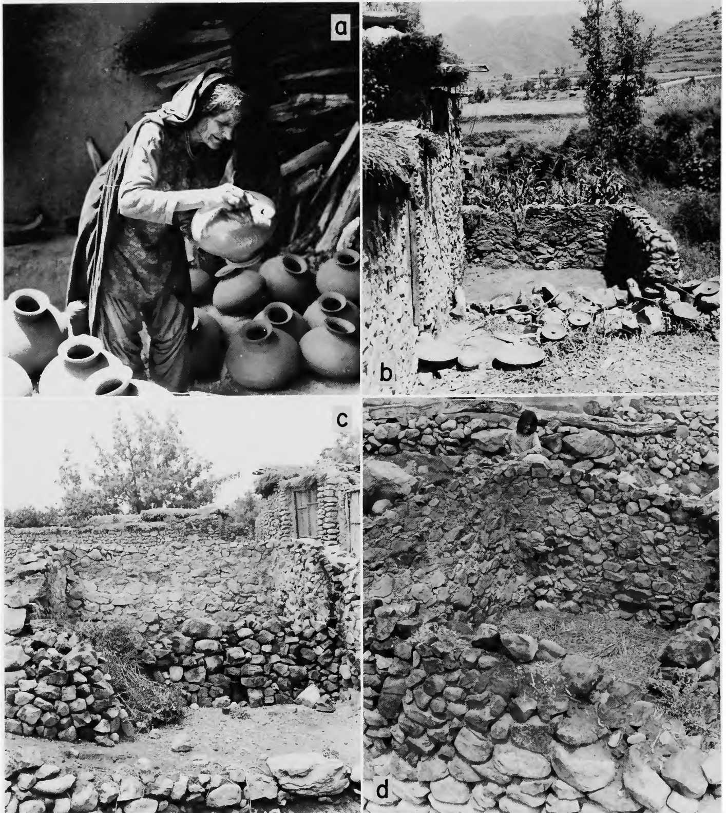
PLATE 19.—Slip application and kilns, Swat, NWFP: a , applying red slip to a water pot with a cloth saturated with the slip; b , open kiln, village Chamthale, upper Swat Valley (height of walls approximately 1 m); c , d , two views of open kiln, Alam Ganj, Swat (height of walls 1.5 m, lower front wall 0.8 m).
