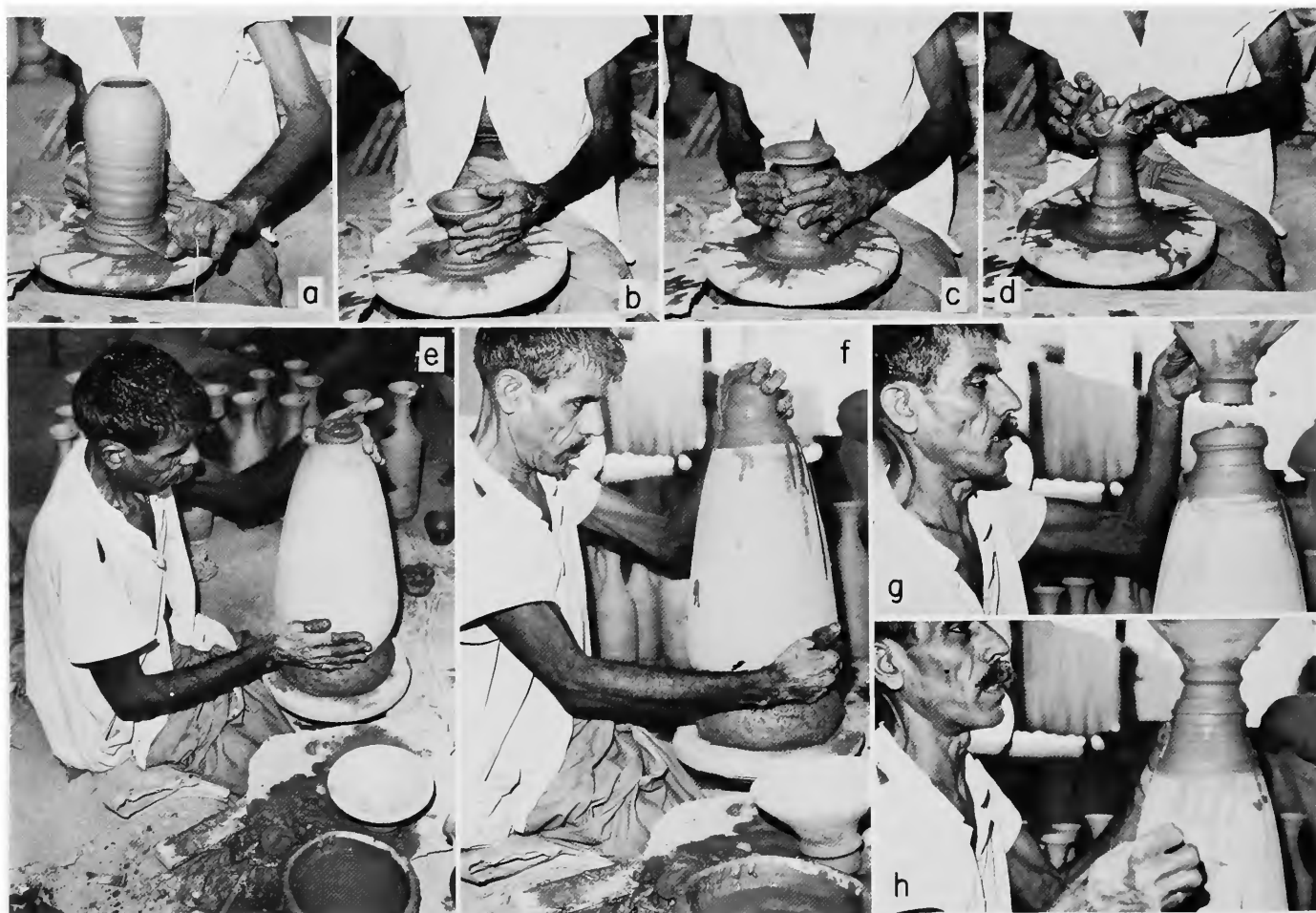
PLATE 71.—Forming a vase in sections, Multan, Panjab: a , throwing the main body of the vessel (here vessel is being cut off with a thread before removal from the wheelhead); b , forming pedestal foot for vase; c , d , forming neck and rim of vase; e , f , joining foot of vessel to main body and attaching main body to the wheelhead in a clay chuck; g , h , attaching neck and rim section by the same method.
