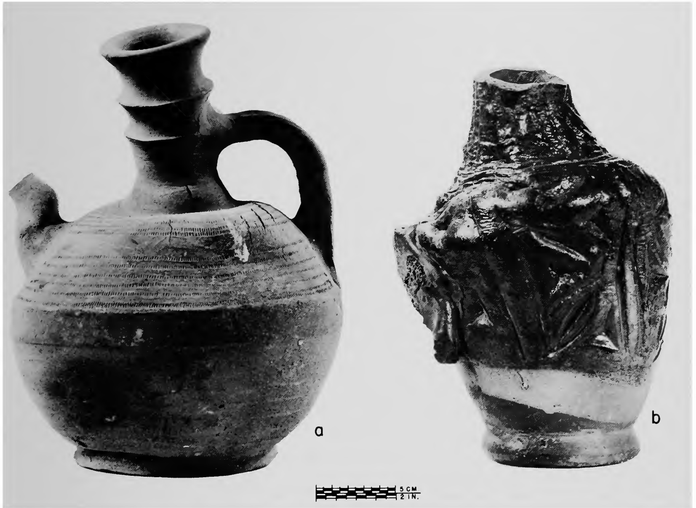
PLATE 82.—Overfired vessels: a , kūzā Shahbaz Ahmed Khel, NWFP (USNM 417,268), fired to olive green color (unglazed), note distortion at shoulder, cracking; b , cilam , Zakhel Bala, NWFP (USNM 417,313), extensive bloating and fusion on one side, neck broken off, green lead glaze changed to bright red (copper red) in the most overfired areas, indicating reduction on those areas, green color retained on other parts.
