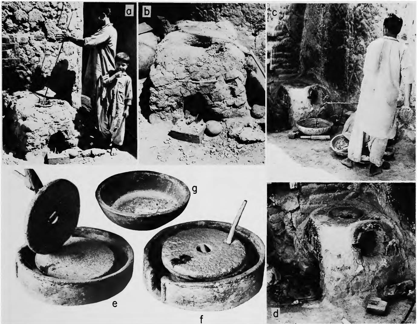
PLATE 60.—Glazemaking, Zakhel Bala, NWFP: a , Hassan Din, with his son, demonstrating how molten lead is stirred in a lead roasting furnace; b , closeup of furnace, overall height about 0.5 m, stokehole for fuel at front, top opening for placing lead in fixed crucible and for stirring and removing lead oxide; c , frit furnace for fusing lead glaze frit, Hassan Din demonstrating how molten frit is scooped out of crucible with iron ladle and poured into water; d , closeup of frit furnace, stokehole lower left, observation and removal opening front right, charging hole at top (sealed when the furnace is in use); e , f , quern (handmill) used to grind frit and other glaze materials, grinding stone (raised in e ) 0.5 cm diameter; g , crucible removed from frit furnace, with some frit still in it (diameter 35 cm, made from normal pottery body).
