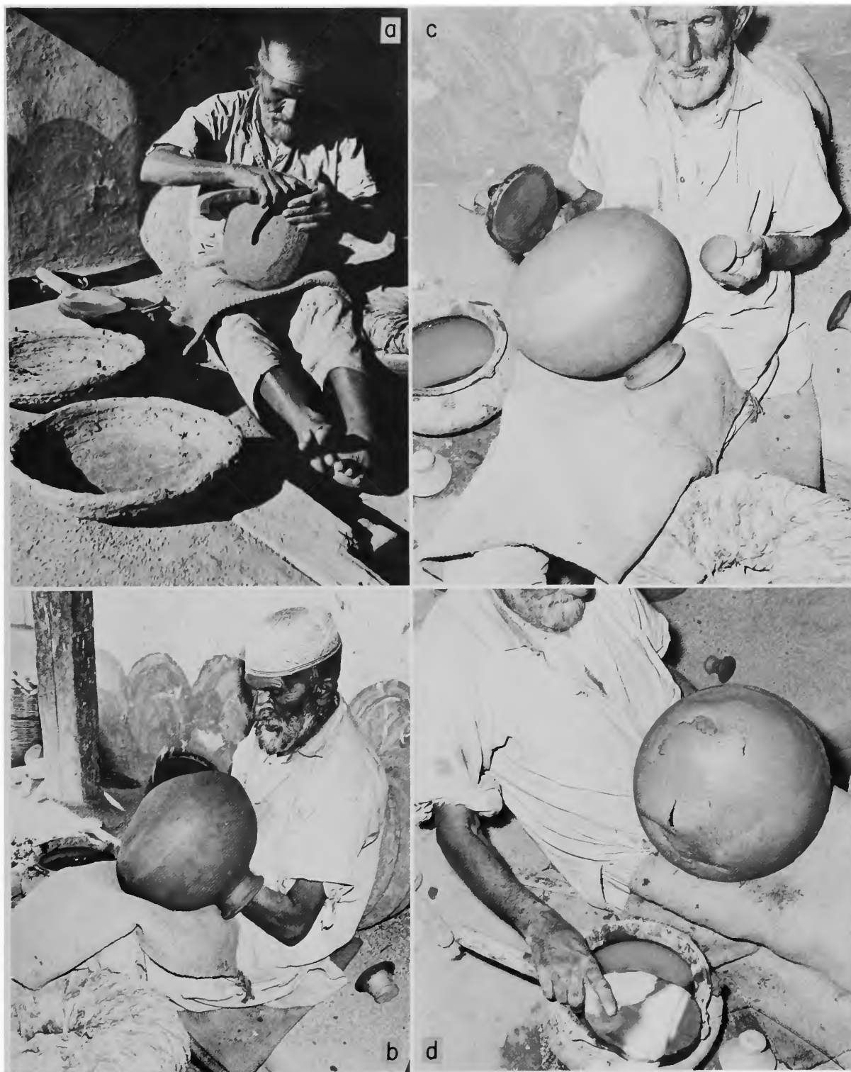
PLATE 16.—Using paddle and anvil to complete the base of water pots, Dir, NWFP: a , trimming off excess clay with a knife before beginning beating; b , forming with paddle and anvil; c , completed form of waterpot; d , cracks appearing in base of vessel during beating are repaired with plastic clay which is blended into the form by further beating.
