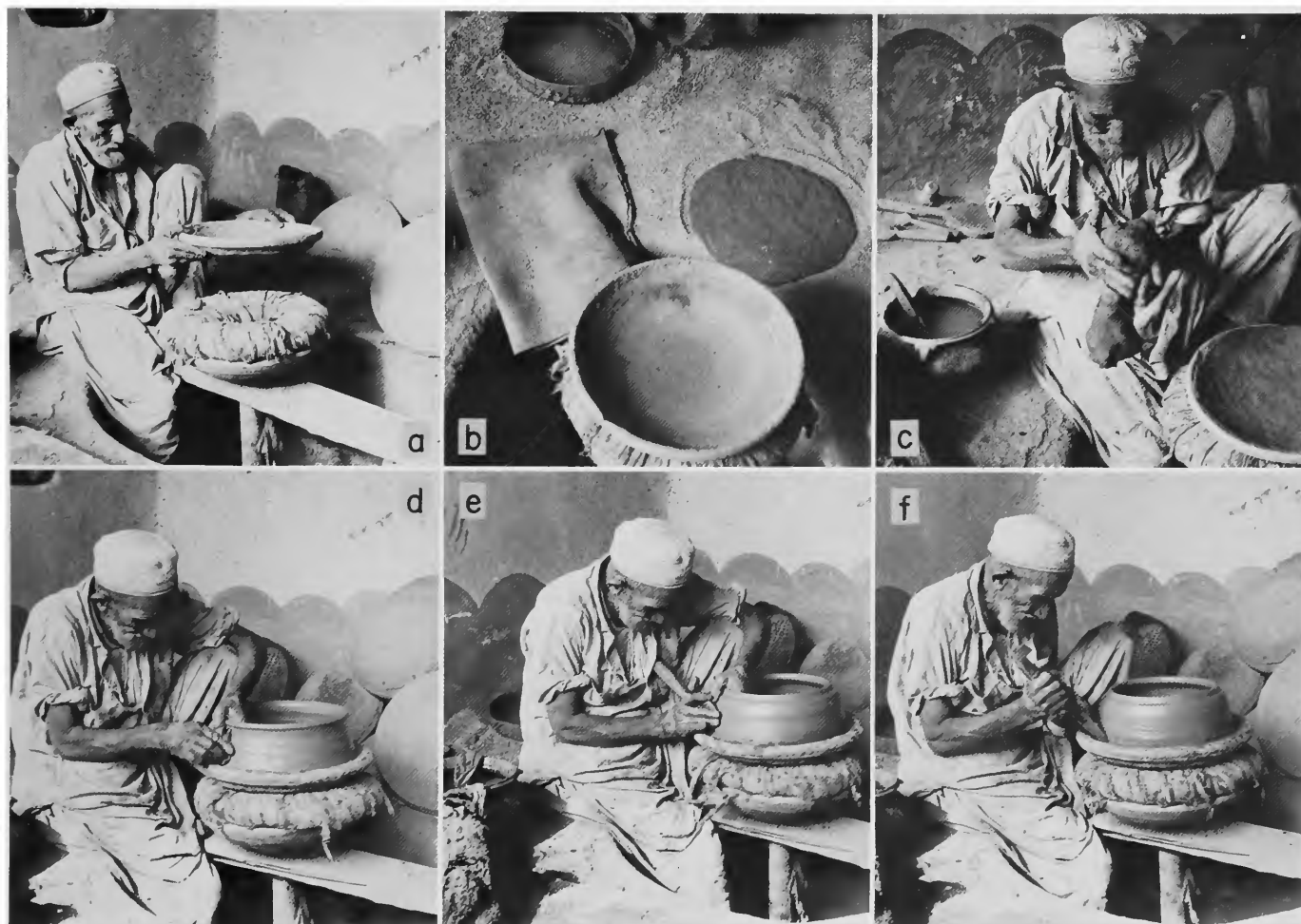
PLATE 14.—Forming vessels on the pit-wheel, Dir, NWFP: a , placing fired clay base mold on cloth pad on the wheelhead; b , mold on wheel (base of vessel has been formed on sand, right back); c , forming coil (note clay for base of vessel to be formed has been placed in base-mold); d , throwing upper walls of a vessel; e , using smoothing tool to refine walls of vessel; f , trimming excess clay from base of vessel, at junction with mold.
