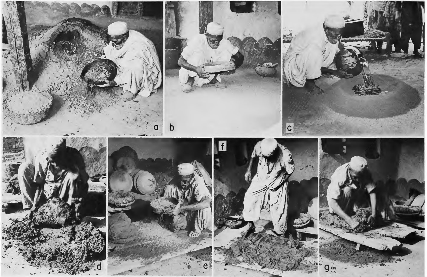
PLATE 13.—Body preparation of vessel, Dir, NWFP: a , potter Khan Zada sieving clay; b , sieving coarse sand onto floor so wet clay will not stick to it; c , pouring water into hollowed pile of mixed clays; d , roughly compacting plastic body; e , sieving sand onto clay preparation bench; f , foot-kneading clay body (note that sand becomes mixed into the body); g , rolling kneaded clay into one lump.
