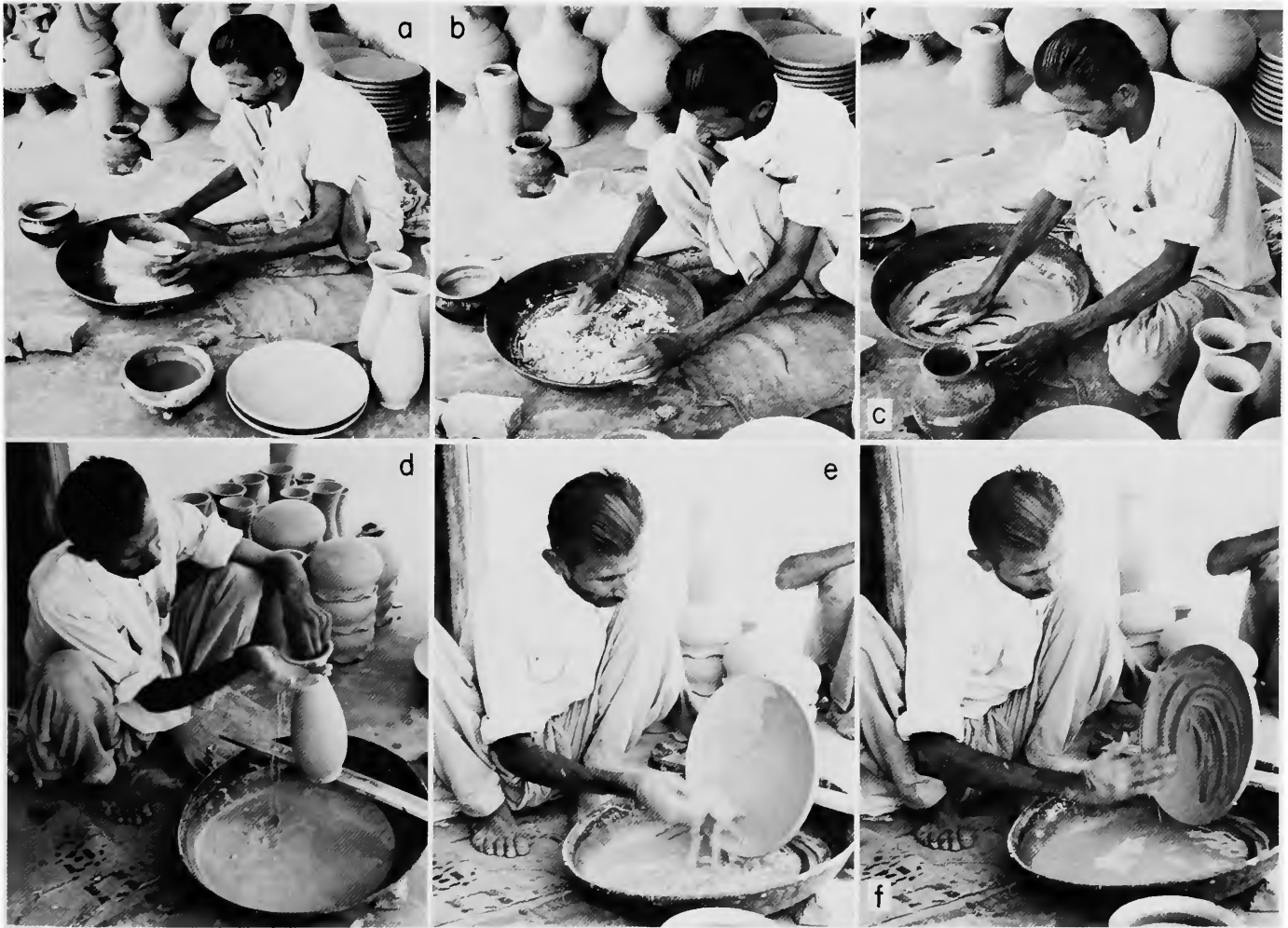
PLATE 72.—Slip application by master potter Khuda Baksh, Multan, Panjab: a , sieving ground slip, b , mixing flour glue with slip powder; c , thinning the slip with water; d , applying slip to a vase by pouring with the hand; e , splashing first coating of slip on a dish; f , first coating being rubbed off and a second coating of slip to be applied.
