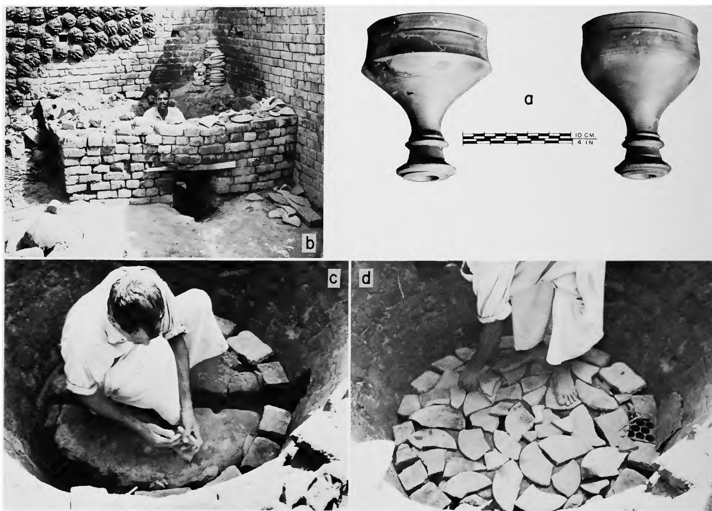
PLATE 35.—Kiln setting and unglazed earthenware by potter Sardar Mahommed, Garhi Maqbulabad, Gujrat: a , topi decorated with red slip (USNM 417,246-B & C); b , Sardar Mahommed setting the kiln; c , placing tiles over air access channel at base of kiln; d , layer of flat sherds placed over air channels at base of kiln. (See Plate 36.)
