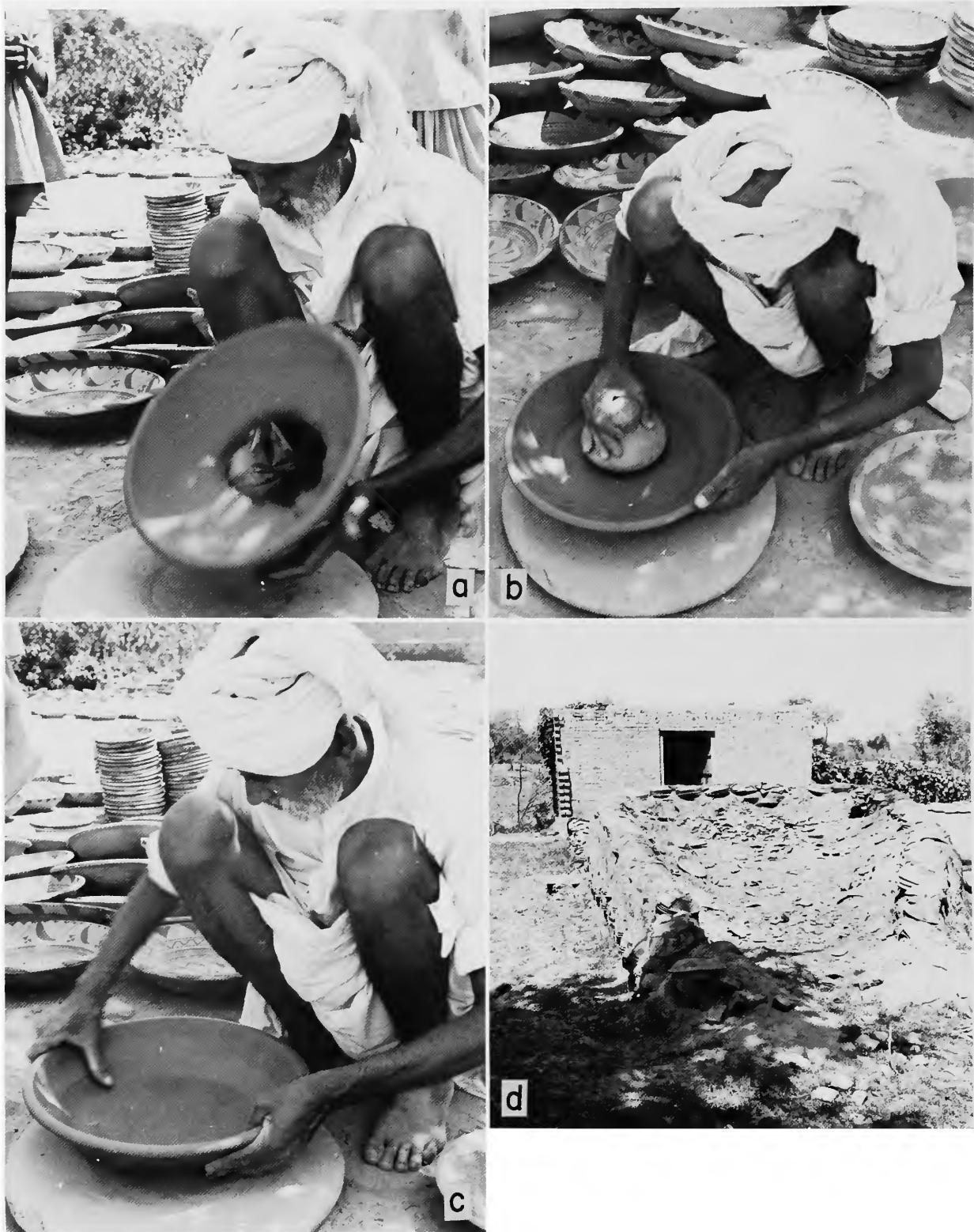
PLATE 39.—Potter Ala Dita completing a dish, Shadiwal, Gujrat (continued): a , squeezing clay from thick sides of thrown form inwards to close the hollow base; b , smoothing base by beating with an anvil; c , hand-smoothing the dish; d , typical open pit-kiln at Shadiwal.
