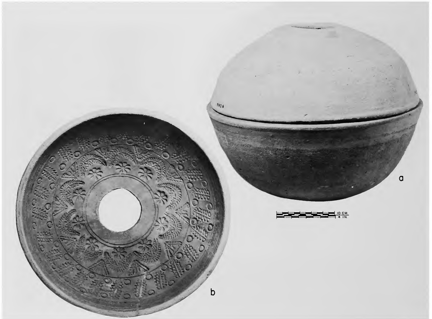
PLATE 67.—Mold used for forming water jars, Zakhel Bala, NWFP (USNM 412,416): a , two parts of mold assembled; b , interior of top mold showing central hole allowing access to interior of vessel for joining two halves of the vessel, and impressed decoration which forms relief decoration on the molded vessel, fired clay. (cf. Plates 21, 22.)
