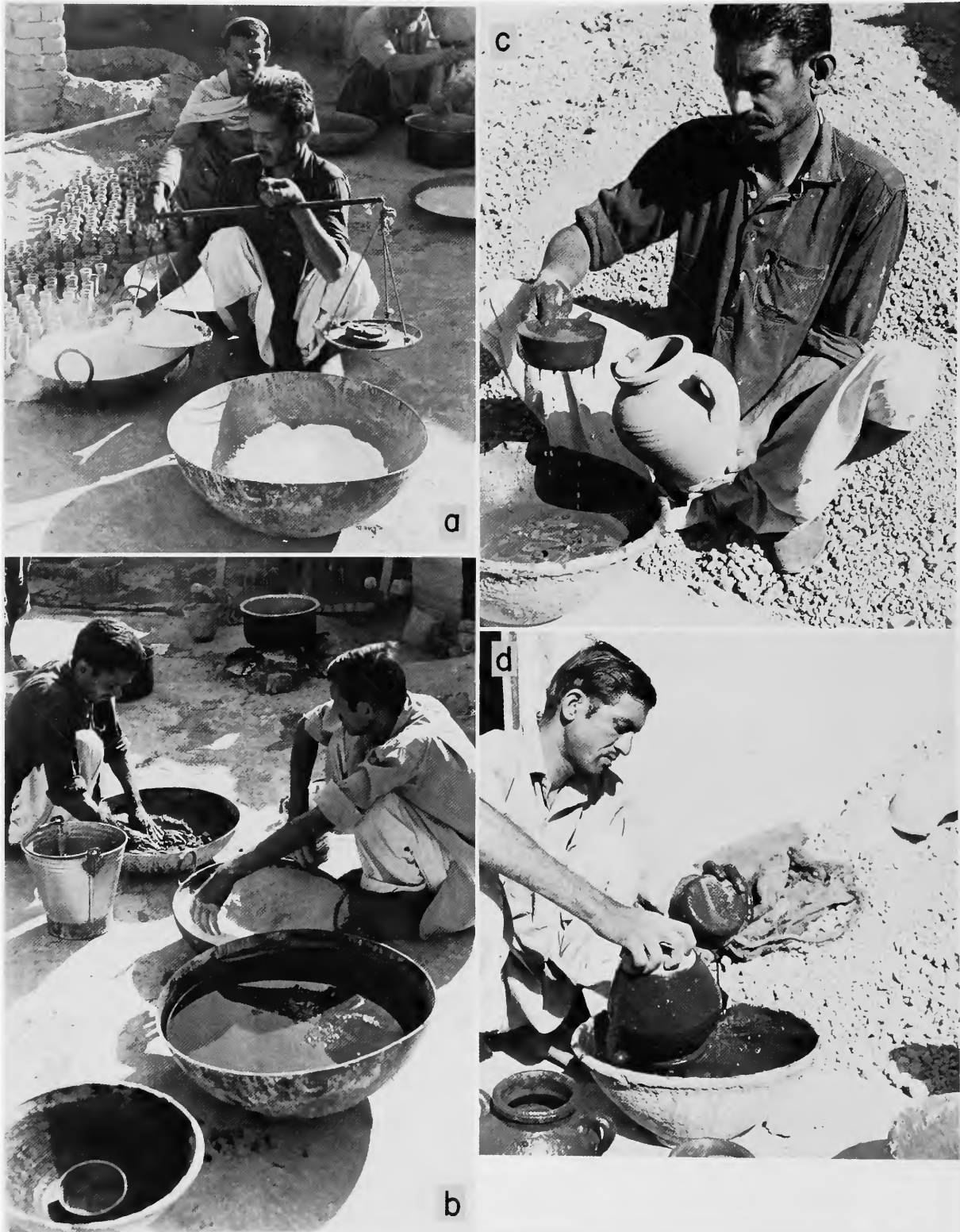
PLATE 51.—Preparing and applying glaze, Quetta, Baluchistan: a , weighing glaze materials; b , mixing glaze in an iron dish; c , pouring glaze into interior of urn (excess glaze is poured from the vessel back into the large bowl of glaze); d , pouring glaze over the exterior of a vessel.
