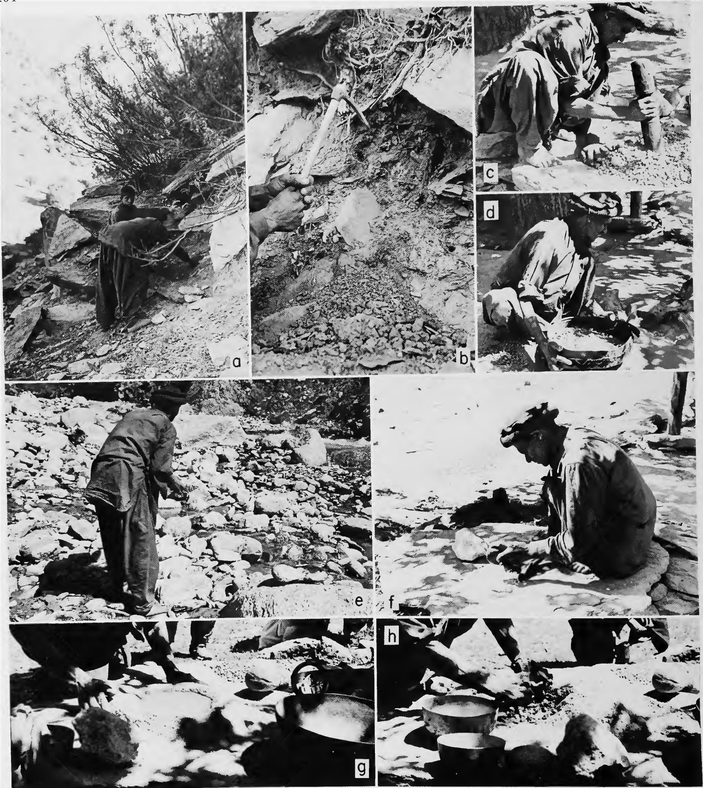
PLATE 2.—Materials gathering and preparation, Bomboret Valley, NWFP: a , general view of clay-digging site; b , digging clay and weathered slate fragments; c , breaking up lumps of clay with a wooden pestle; d , sieving clay; e , selecting quartz pebbles from bed of Bomboret River; f , crushing quartz using a stone as a hammer, g , adding water to clay in a hollowed pile; h , rough-kneading body.
