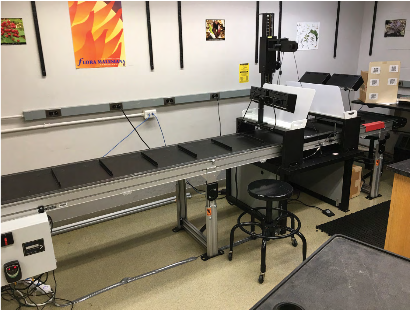
(Above) Apparatus for scanning large quantities of mounted botanical specimens at the National Museum of Natural History (NMNH)
