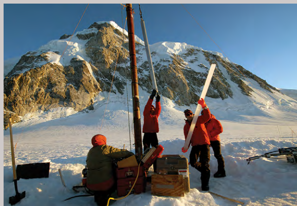
(Above) Extracting cores from an ice sheet (NSF/Doug Clark)
