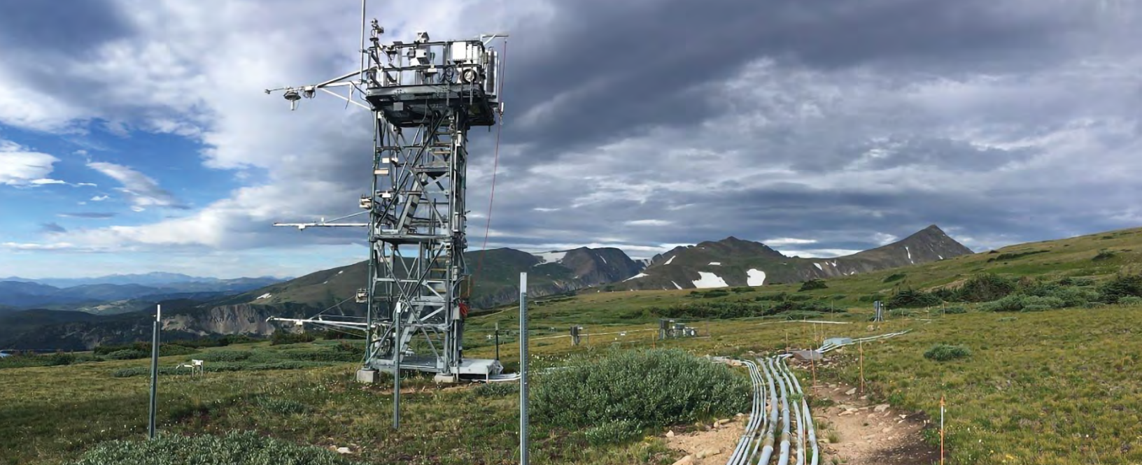
(Above) NEON terrestrial installations, such as the meteorological flux tower shown above, use a broad variety of platforms and technologies to collect data on life, air, soil, water, and climate at field sites. (NEON)
