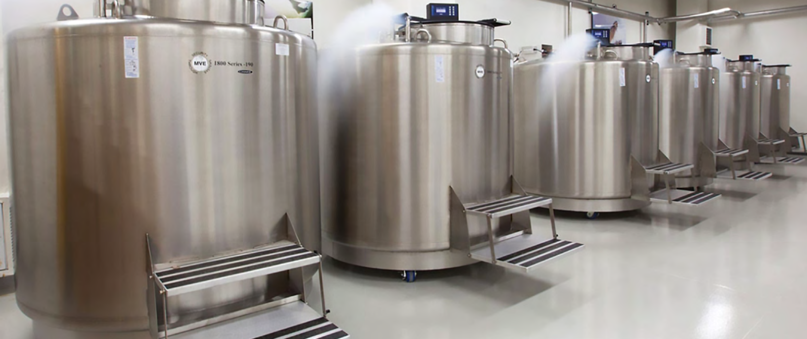
(Above) CBR stores specimens cryogenically in liquid nitrogen freezers. (Smithsonian)
