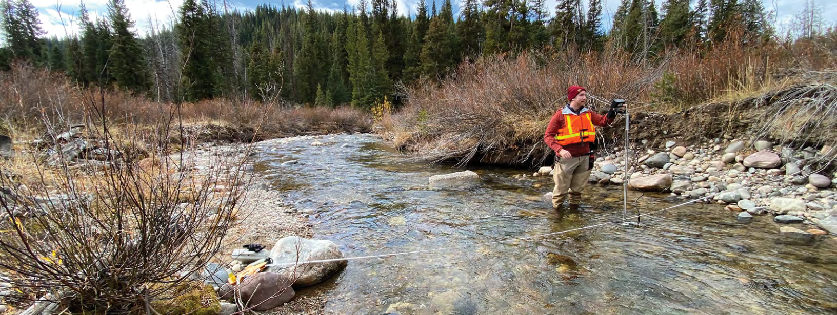
(Above) NWQL hydrologist measuring streamflow, Moran, Wyoming (USGS/Rob Hood)
