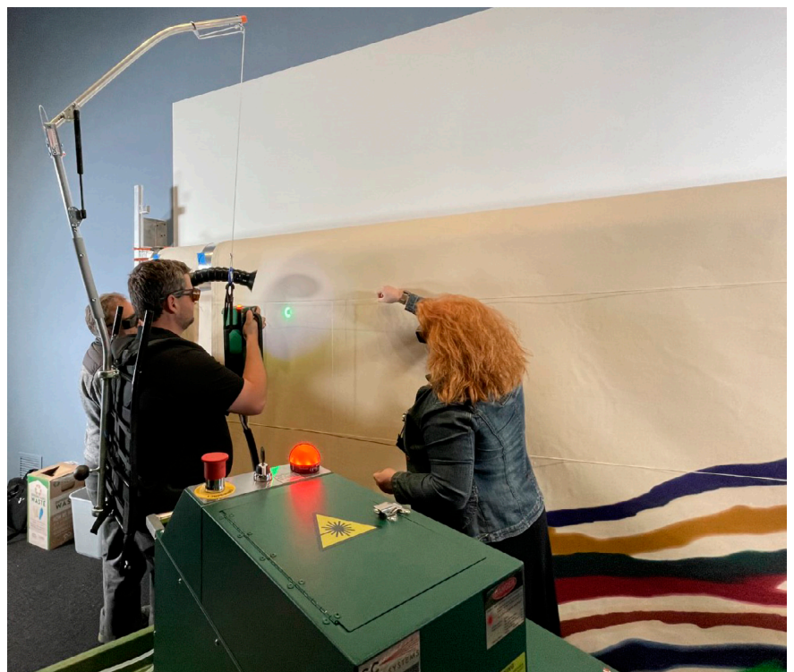
Figure 6. Image taken during laser cleaning of Beta Upsilon showing the suspended canvas, with sectioning twine to guide the cleaning process, and the laser operator's use of a back suspension to control laser application
