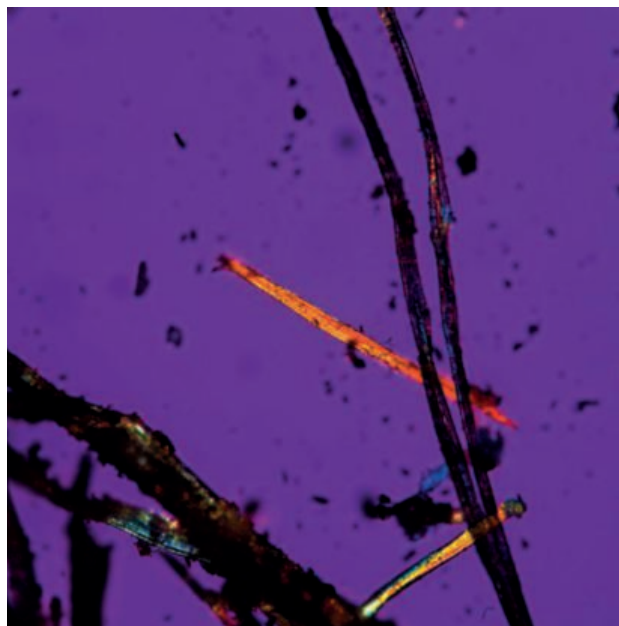
Figure 15. Identification of the hemp fibers was confirmed under the polarized light microscope. Here the fiber is viewed under crossed polarized light with a gypsum plate. It is yellow when turned 90° from extinction.
