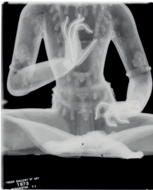
Figure 8. X-ray radiograph of Freer bodhisattva, revealing wire armature in fingers.
