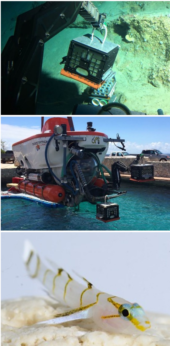
FIGURE 5 Retrieval of a FARMS unit on the slope of Curaçao using the Curasub submersible and its hydraulic arm, and the second-known specimen of Psilotris laurae , collected in the FARMS deployed at 146 m. Top and middle photos by C. Baldwin, bottom by Barry Brown.
