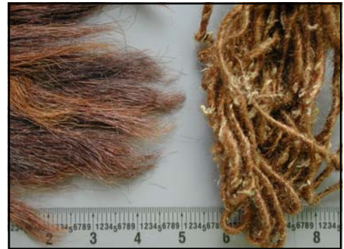
On the left unprocessed beard of byssus (dry state), Algiers. On the right, z-twist-spun single yarn of byssus, Italy, 1965.
