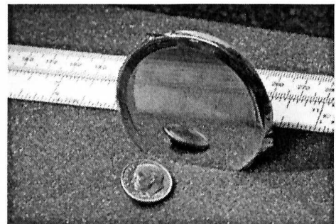
One of the new infrared filters, hand-mounted on a metal support ring. Optical light is partially transmitted by the thin film; infrared wavelengths are blocked, except over a narrow range.
