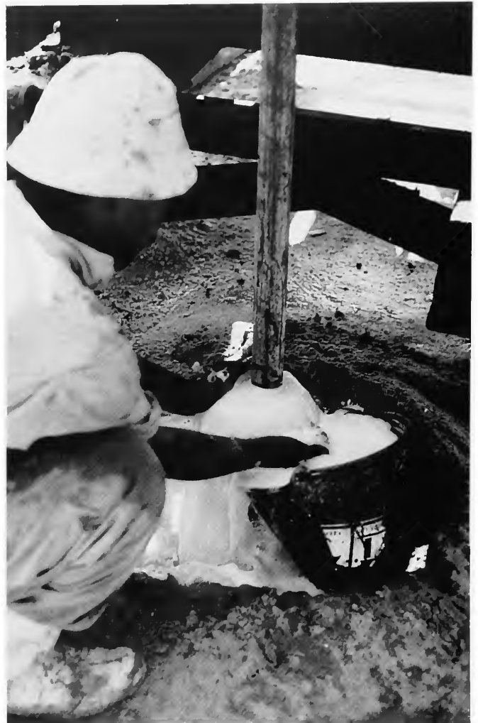
FIGURE 6.—Drilling through consolidated carbonate section of late Pleistocene age in the region west of Alexandria. Pumped water is typically white when circulated through drilled carbonate sequences. Photograph taken at site S85 in September 1990.
