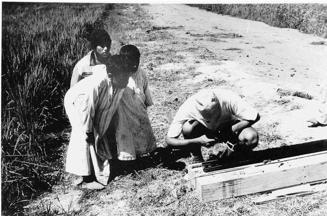
FIGURE 8.—After extraction from the drill barrel, mud-rich sediment cores are cut into 5-foot (1.5 m) lengths, placed in plastic liners, and described prior to storage in boxes. Photograph taken at site S55 in September 1989.
