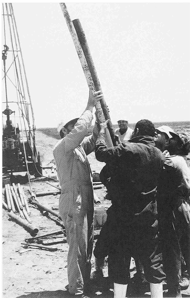
FIGURE 7.—Mud-rich sediment core of Holocene age placed in a plastic liner after extrusion from the drill barrel. Photograph taken at site S18 in April 1987.
