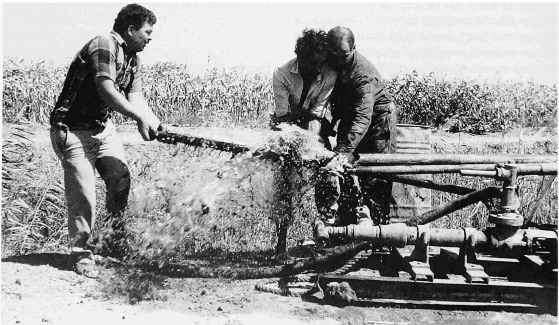
FIGURE 4.—Extrusion from drill pipe of stiff clayey silt of late Pleistocene age, using high pressure pumping of circulated water. Photograph taken at site S55 in September 1989.
