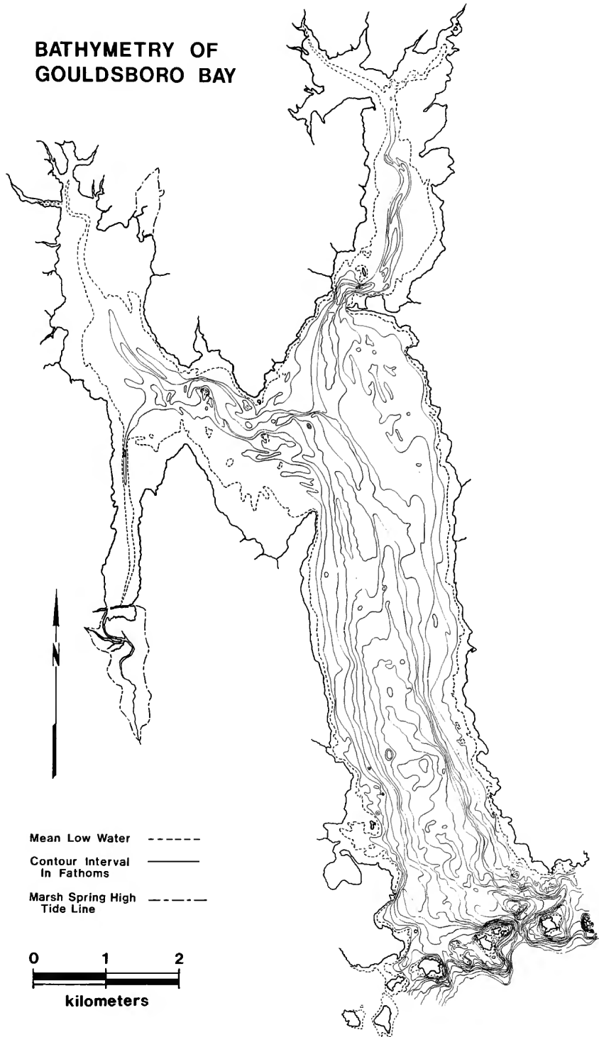
FIGURE 3.—Bathymetry of Gouldsboro Bay (contoured from National Oceanographic Survey's original hydrographic survey no. H-1505, conducted in 1881).
