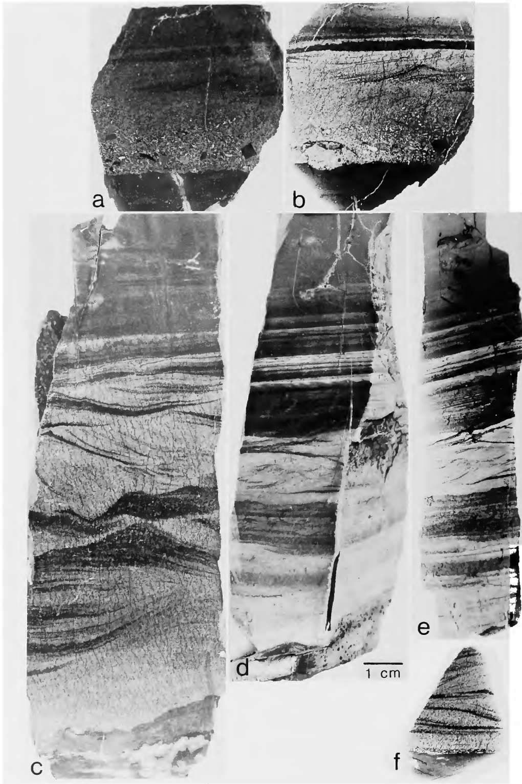
FIGURE 56.—Examples of sharp-based and sharp-topped, graded and laminated layers suggesting multiple depositional origin. a,c,e are polished sections; b,d,f are thin sections. a,b , Graded layer (A division) not followed upward by horizontally layered B division; note, however, upper rippled bedform and sharp top. c-f = Graded layers with erosional base (note small flame structures), and cross stratified throughout; some dark laminations (in d and f ) highlighted by concentrations of heavy minerals. Localities (Figure 2): a-c = site 18; d,e = site 19; f = site 52. Scale bar applies to all components.
