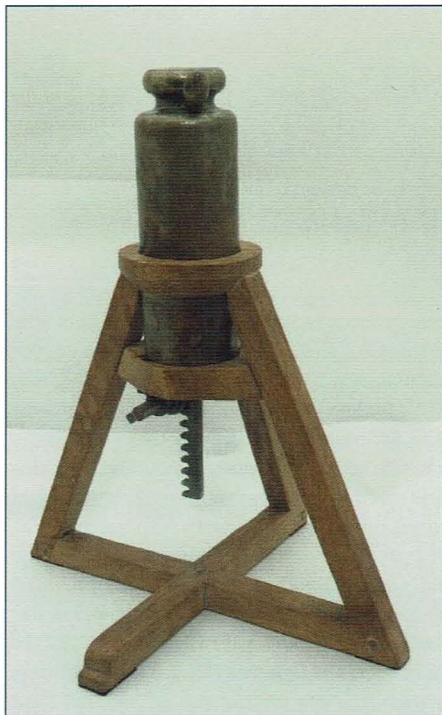
Fig. 2 (a) The first functioning British air pump —produced by Robert Hooke, working with and for Robert Boyle, in Oxford in the late 1750s—no longer exists. This roughly half-sized replica was made from Boyle's published description and illustration. The picture was taken without the globe [PH.314816]; and (b) Engraving of the original air pump from Robert Boyle, New experiments physico-mechanical, touching the air (Oxford, 1660).
