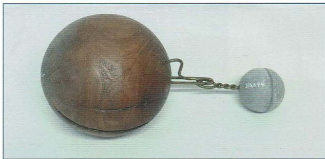
Fig. 4 Robert Hooke presented his first depth finder to the Royal Society in September 1663, at a time when several founding fellows were discussing ways to improve oceanic navigation. Correspondence in the accession file indicates that Eichner made this replica to look 'weather beaten and aged.' [PH.316644].
