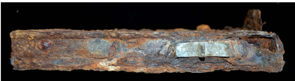
FIGURE 6. Bottom surface of the lock; back is face uppermost. The brass slide at right locked the night bolt (now inside the case, visible below the gap at the upper right) when moved to the right. The flange is in the background, at upper right.
