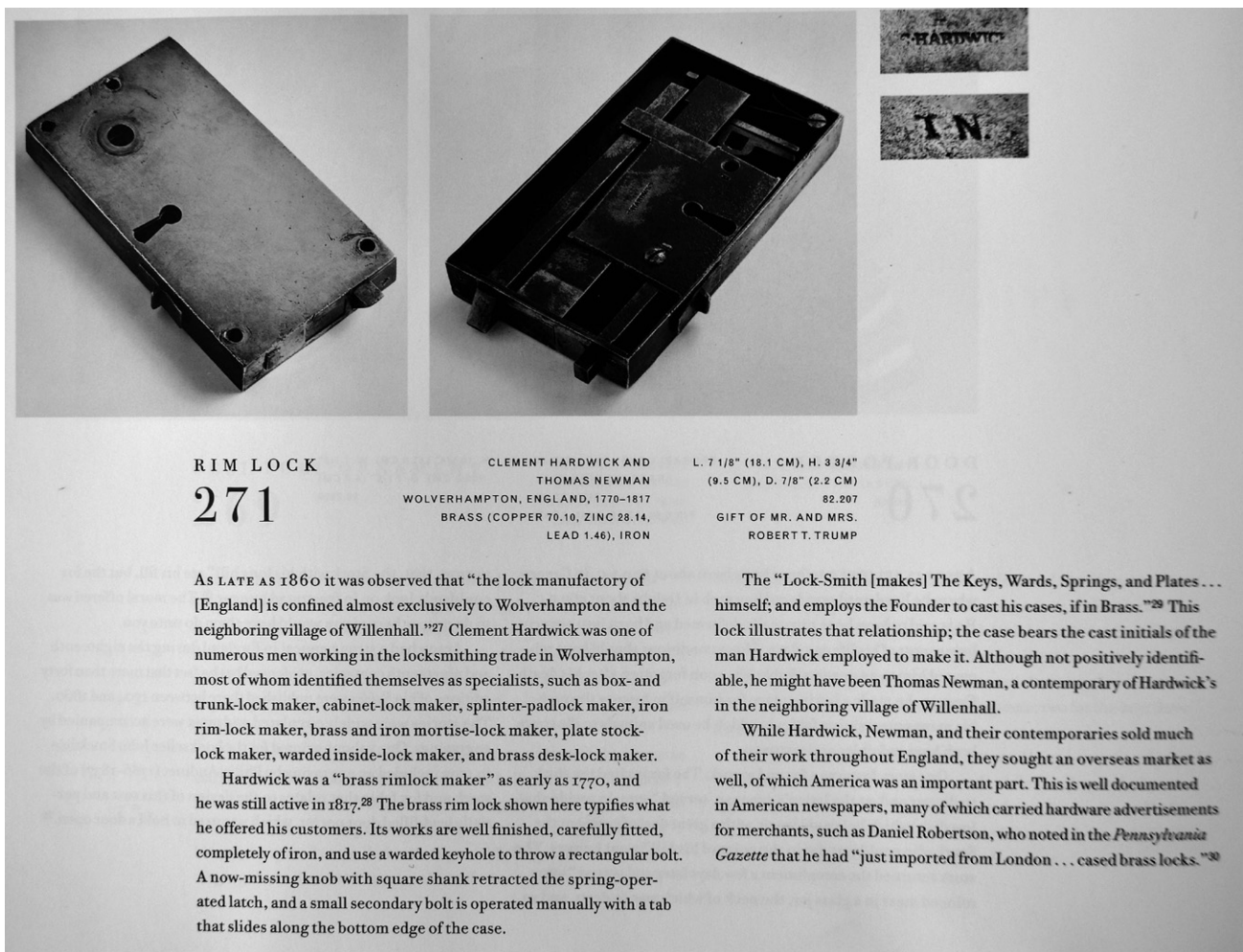
FIGURE 13. Brass rim lock, late eighteenth–early nineteenth century, made by Clement Hardwick and Thomas Newman in England. The slide at the bottom surface of the lock and the aperture allowing up-and-down movement of the latch are similar to those on SERC's lock.
