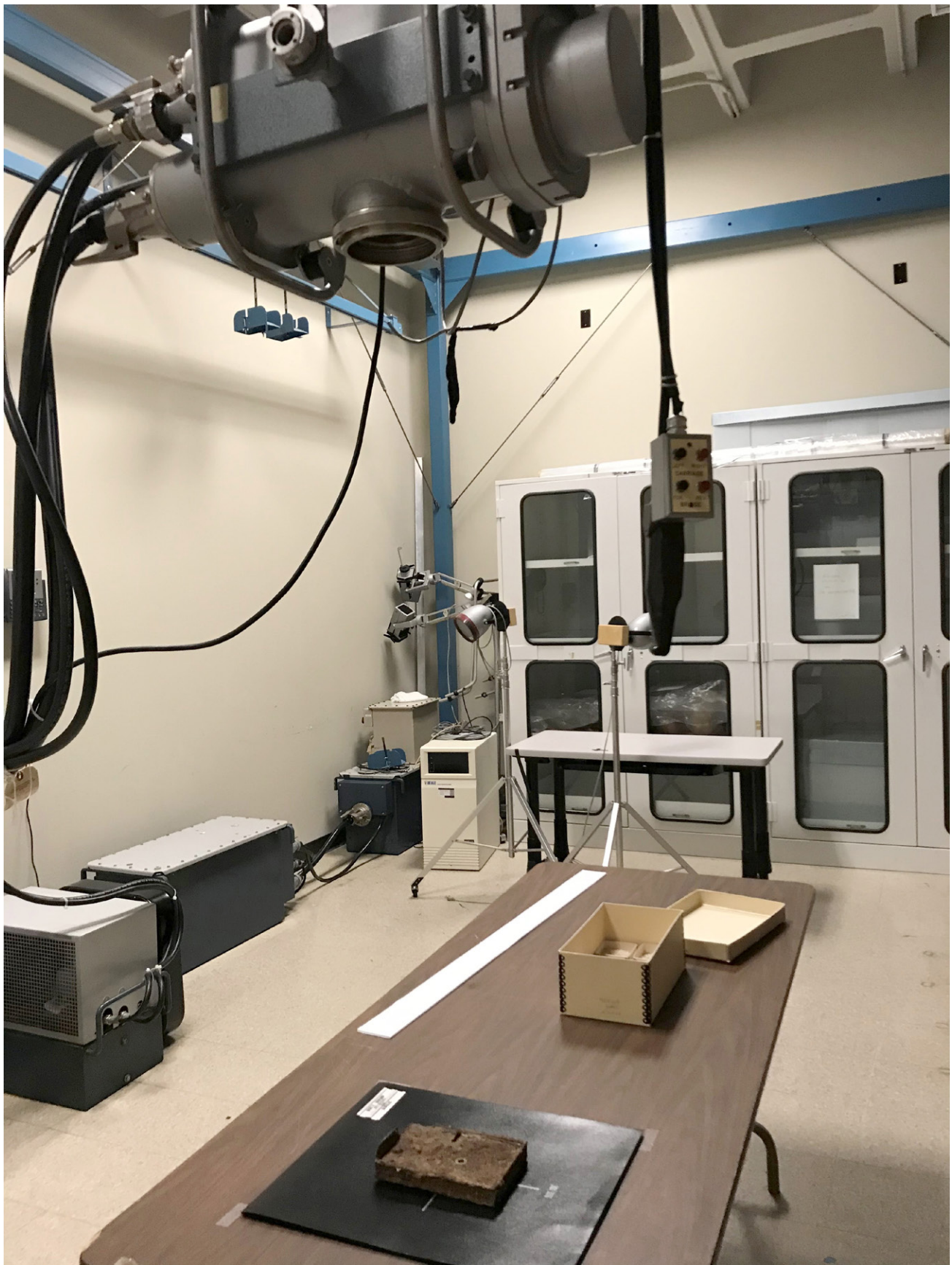
FIGURE 25. The Philips MG320 X-ray unit used for the digital radiography of the box lock.
