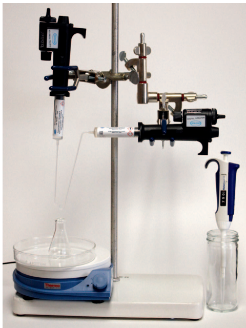
Figure 1. Setup of equipment for sodium sulfite titration method. (© I. Finkelde.)
