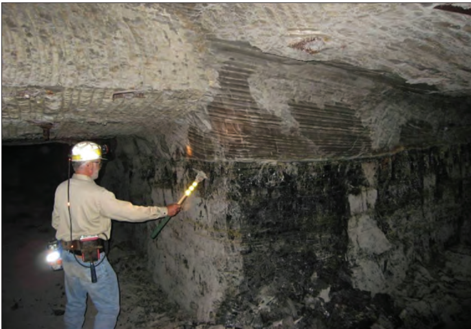
Figure 16 Photograph showing rhythmic lamination in sandy facies of the Dykersburg Member in the Millennium Mine, with lamination offlapping the top of the coal. Sediment thus was deposited in a wedge, prograding from left to right.
