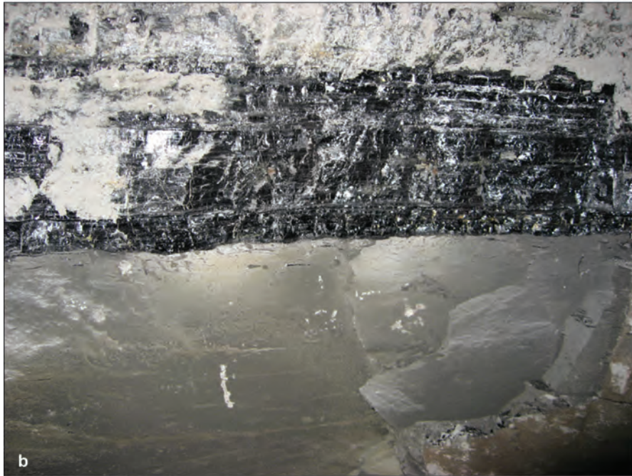
Figure 21 Photographs of siltstone “splits” in the Springfield Coal. (a) Upper “bench” of coal splitting into multiple layers, with ragged splaying of lower coal layers at the Millennium Mine. (b) Contact between the upper coal bench and a massive siltstone split in American Coal’s Millennium Mine, approximately 0.6 mi (1 km) west of the main Galatia channel. Notice the complete absence of root traces in the siltstone.
