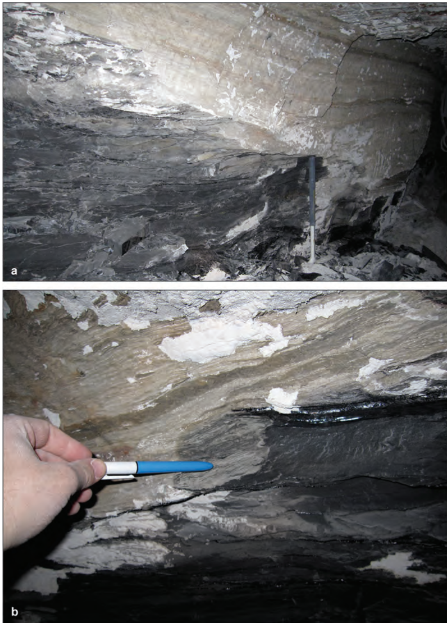
Figure 13 Photographs showing the ragged, erosive contact between the light-colored siltstone of the Dykersburg Member and the underlying coaly shale of the Galatia Member in the channel crossing at the Galatia Mine, Saline County, Illinois. (a) View of the east wall of the entry. Coaly shale of the Galatia Member grades laterally northward (left, out of view) to shaly Springfield Coal. The pick is approximately 2 ft (60 cm) long. (b) Close-up view on the west wall of the entry. The heart of the Galatia channel is south (left) of view. Notice how erosion undercut the clay below layers of tough, fibrous peat.
