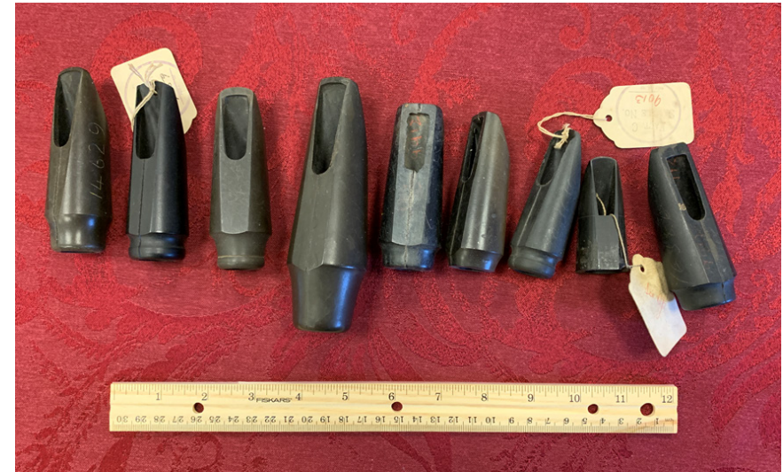
FIGURE 3. Hard-rubber mouthpiece castings made by the American Hard Rubber company in the 1920s. Note the longitudinal line on most of the mouthpieces, indicating that they were cast in a multi-piece mold. Image by Jesse Bross; courtesy of the Butler Museum, Butler, New Jersey.
