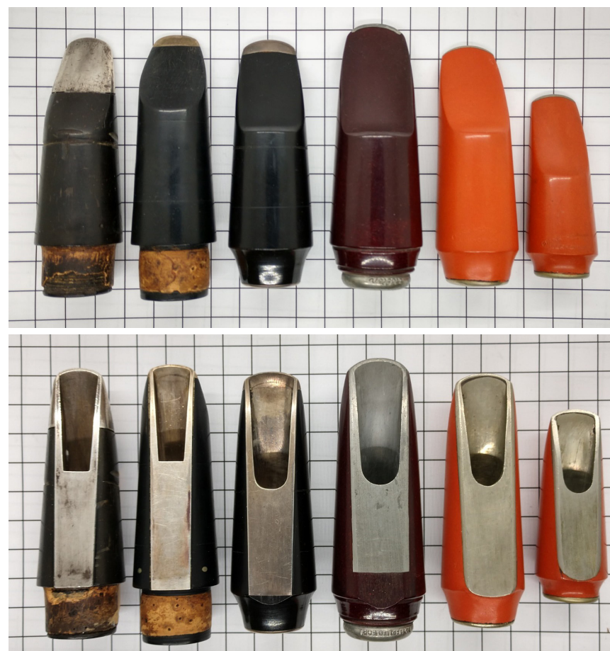
FIGURE 8. At top, six hard-rubber mouthpieces with metal cores and tables; below are opposite sides of the same. From left are three with silver cores and tables: an unmarked clarinet mouthpiece closely matching the 1905 Starke patent drawing, an Arthur Goldbeck clarinet mouthpiece, and an unlabeled alto closely resembling the Goldbeck clarinet mouthpiece design.
