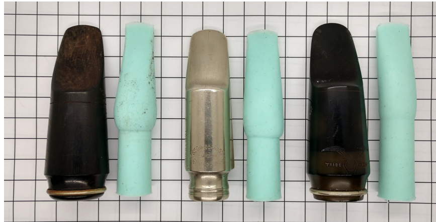
FIGURE 2. Wood, metal, and hard-rubber mouthpieces paired with silicone-rubber casts of each interior cavity. From left, an unbranded wood alto; Goldbeck Superb nickel-silver alto; Conn eagle trademark hard-rubber alto. The casts show the exact shape of the respective large chambers. Gridlines in the background of this and subsequent images are one centimeter apart. Author's photo.
