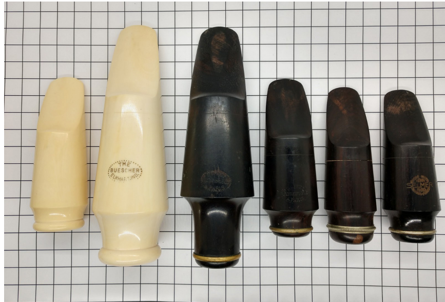
FIGURE 4. Saxophone mouthpieces made from natural materials. On the left are two ivory mouthpieces. The smaller one has the telltale grain of modern or fossil elephant ivory. The larger mouthpiece for baritone, labeled “THE BUESCHER,” lacks the indicative elephant ivory grain. A tiny chip removed from the inside of the mouthpiece, examined in an analytical scanning electron microscope, confirmed it is ivory. Judging from the characteristics of the non-elephant ivory and from its size, the mouthpiece was likely made from a hippopotamus incisor.
