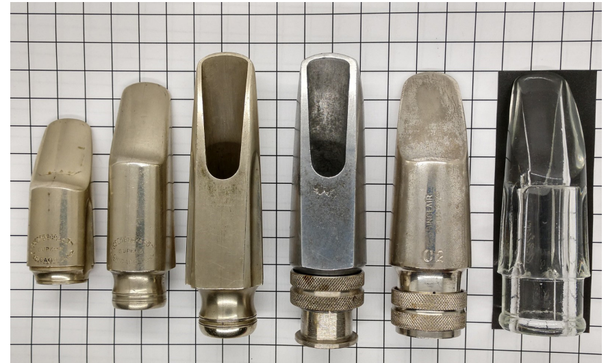
FIGURE 10. Early saxophone mouthpieces of metal or glass. From left, three made by Arthur Goldbeck of nickel silver, cast in two halves and silver-soldered together; mouthpieces of aluminum, and of silver plate over nickel silver, both by the Sinclair Company, with the adjustable shank mechanism patented in 1920. At right, a glass (crystal) mouthpiece for c-melody, made by O'Brien, possibly after 1930. Author's photo.
