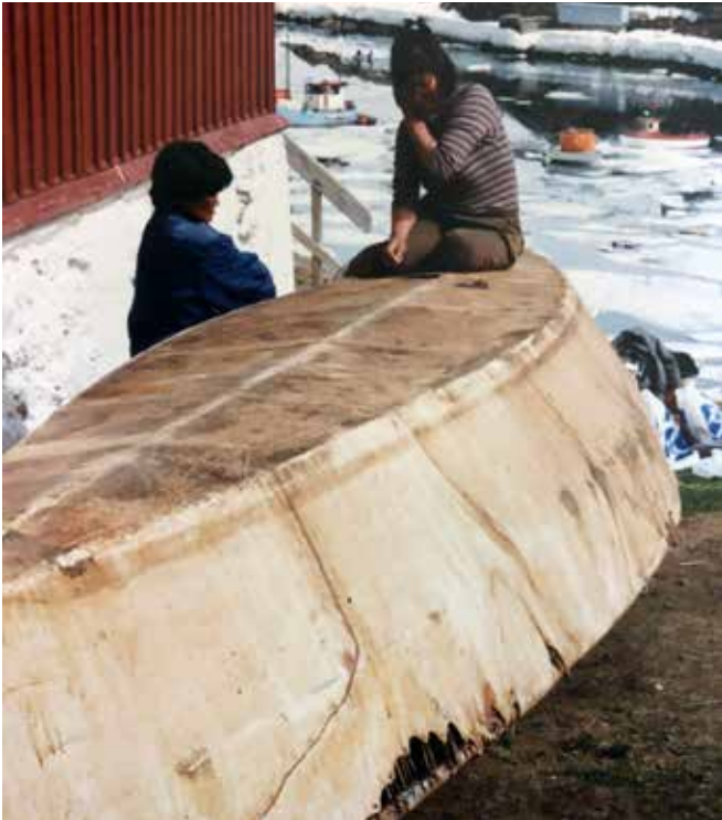
The umiaq with new skins almost completed, gunwale lashings shown, and a "tsakker" (ulu) resting on the boat bottom. Photo by Sheila Romalis
