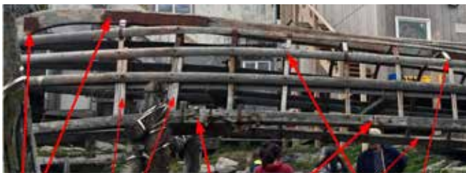
The stern of the same boat shows a supplemental reinforcing block lashed onto the original frame. Nylon rope laces the hides to the frame. Plastic cord became common in the Bering Sea during the 1970s. Photo by Richard D. Mohr, July 2017
