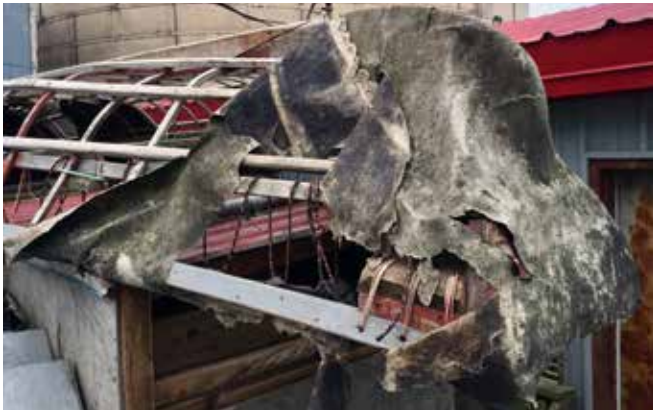
The stern of the same boat shows a supplemental reinforcing block lashed onto the original frame. Nylon rope laces the hides to the frame. Plastic cord became common in the Bering Sea during the 1970s. Photo by Richard D. Mohr, July 2017
