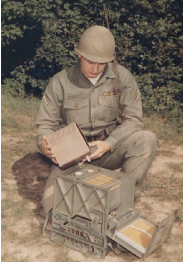
Figure 8. A soldier refuels a 300 W hydrazine fuel cell, ca. 1964. Courtesy of the US Army Mobility Equipment R&D Center.
