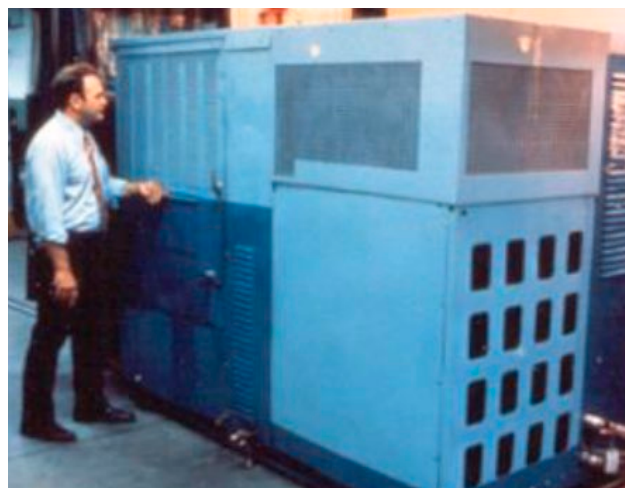
Figure 13. UTC 40 kW model PC-18 phosphoric acid fuel cell, 1979. Courtesy of the US Department of Energy.
