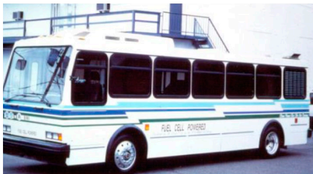
Figure 16. H Power phosphoric acid fuel cell bus, 1996. Courtesy of the US Department of Energy.
