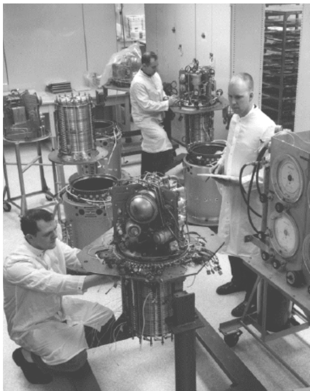
Figure 10. Apollo fuel cell assembly at Pratt & Whitney. From the Science Service Historical Images Collection, courtesy Pratt & Whitney.
