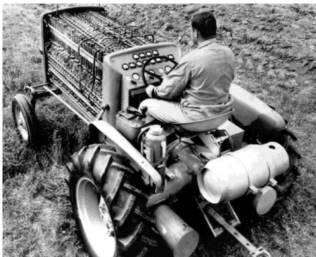
Figure 6. Allis-Chalmers fuel cell tractor, 1959. From the Science Service Historical Images Collection, courtesy Allis-Chalmers
