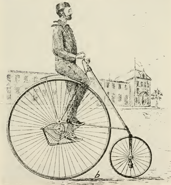
a , Lallement velocipede of 1866. Photograph No. 784-G. b , Star bicycle of the 1880's. Photograph No. 784-H.
