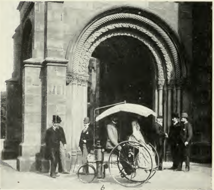
a , Steam-operated velocipede constructed by S. H. Roper in the late 1860's. Photograph No. 36684.
