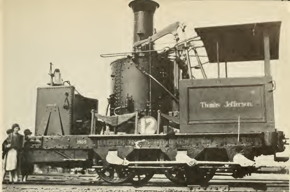
Figure 40.— John Hancock , bearing name Thomas Jefferson , at the Fair of the Iron Horse, September 30, 1927. When first placed in service, "grasshoppers" did not use metal water tanks.
