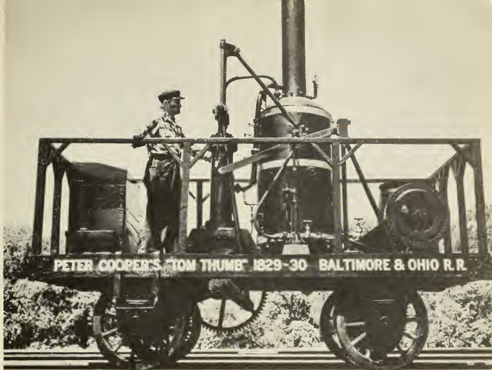
Figure 15.—Full sized operable replica of Cooper's Tom Thumb , built in 1926 by Baltimore and Ohio Railroad Co.
