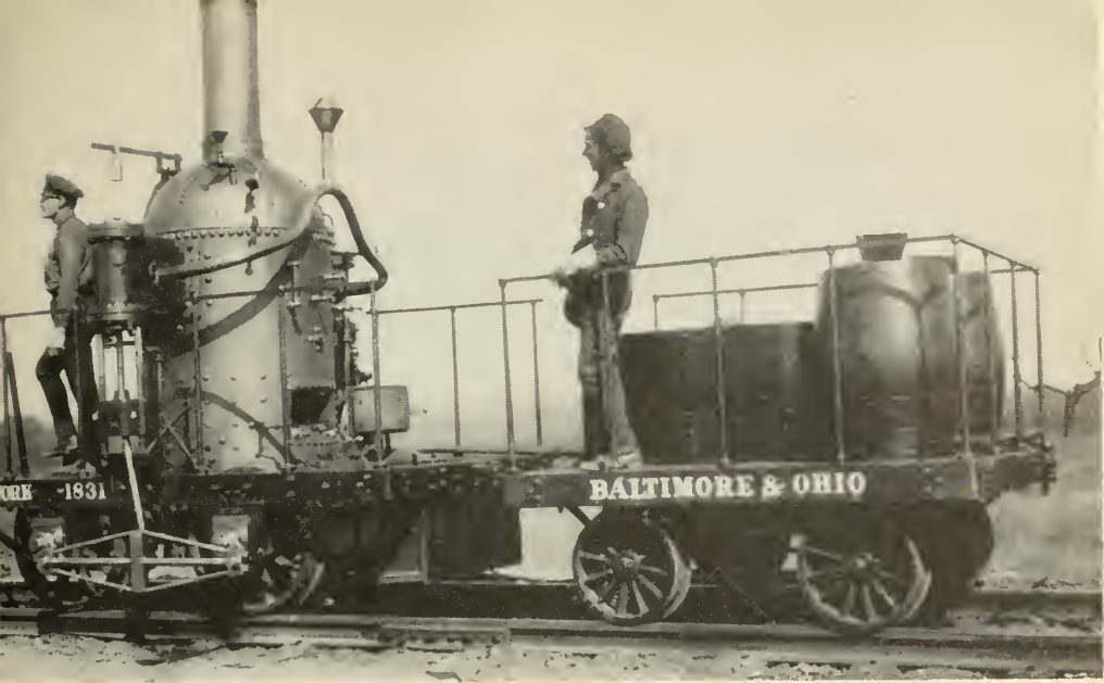
Figure 17. — Full sized operable replica of Davis' York, built in 1927 by Baltimore and Ohio Railroad Co.
