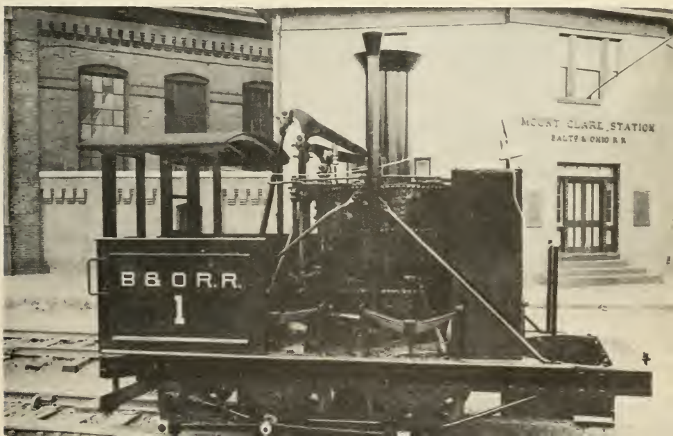
Figure 45.— John Quincy Adams as restored for exhibition at Dayton, Ohio. This is the oldest complete American-built locomotive in existence. Metal water tank is not original.
