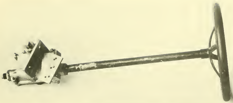
Figure 74.—Steering wheel, column, and gear box of Winton "Bullet No. 1."
