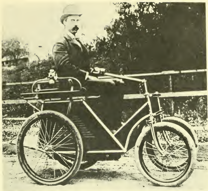
Figure 19.—Stephen M. Balzer with one of his early rotary-engined experimental vehicles.
