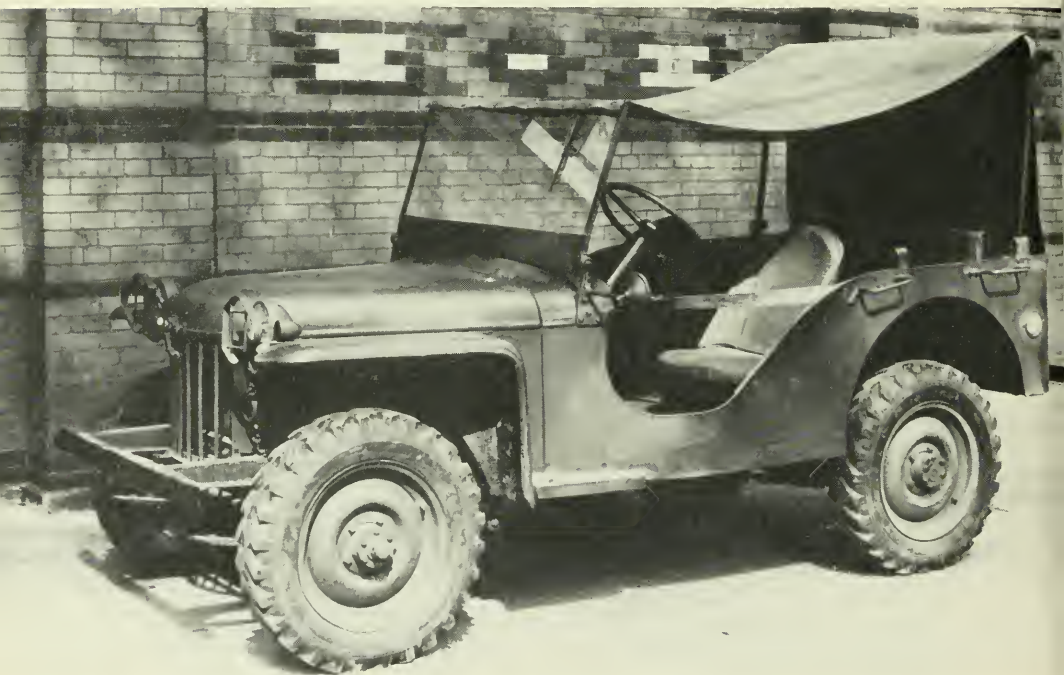
Figure 103.— 1940 Bantam 1/4-ton Army truck, one of a group of 62 prototypes of the world-famous "jeep."
