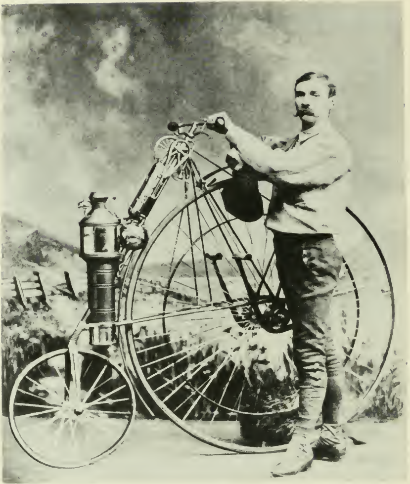
Figure 8.—Lucius D. Copeland and his steam bicycle of the mid-1880's.
