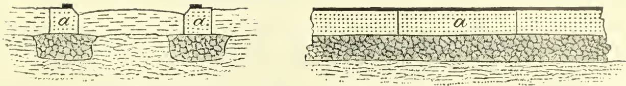
FIGURE 60.—Detail of roadbed of Philadelphia and Columbia Railroad. A few miles of railway consisted of strap iron rails secured to a continuous line of granite blocks (a). From David Stevenson, Sketch of the Civil Engineering of North America (London, 1838).
