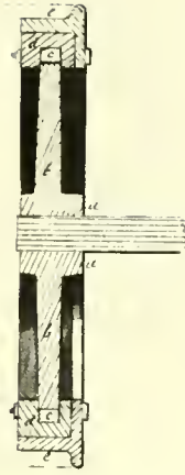
FIGURE 73.—Baldwin's locomotive wheel, showing wooden felloes ( d ) between spokes and rim. From U.S. patent, April 3, 1835, restored drawing. National Archives photograph.
