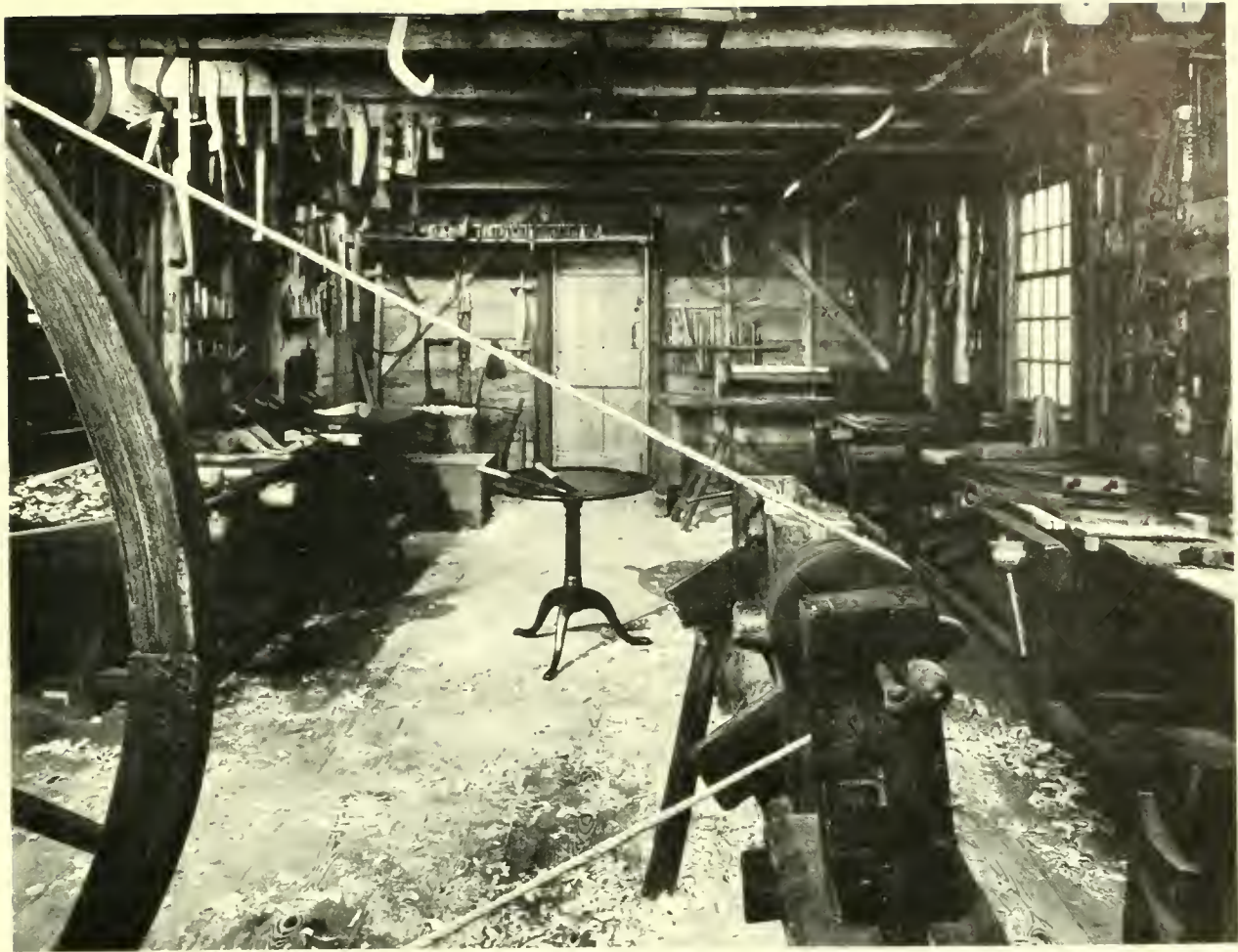
FIGURE 22.—Great wheel lathe (foreground, 1765–1800) and pole lathe (right background, 1750–1765) from the shop of the Dominy family of Easthampton, Long Island, and now installed in the Henry Francis du Pont Winterthur Museum. Note the two spring poles (one in use) at upper right. Photo courtesy of Henry Francis du Pont Winterthur Museum.
