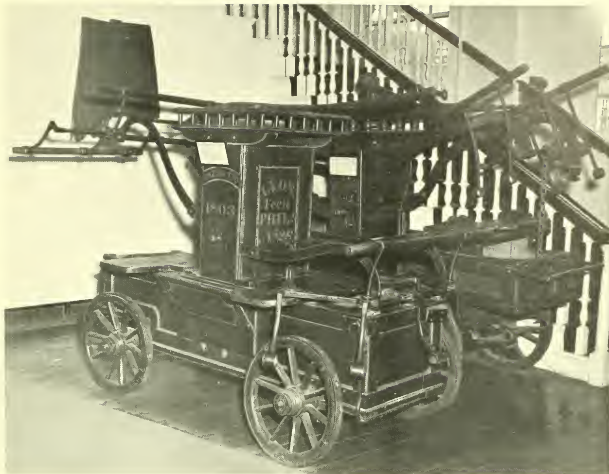
FIGURE 6.—Philadelphia-type fire engines of about 1800, displayed in Independence Hall group. The machine in the foreground is signed by Lyon, and the one in the background is of the same period. Detailed similarities suggest either that Lyon built the second one also or that he supplied the blacksmith-work for it. National Park Service photograph.
