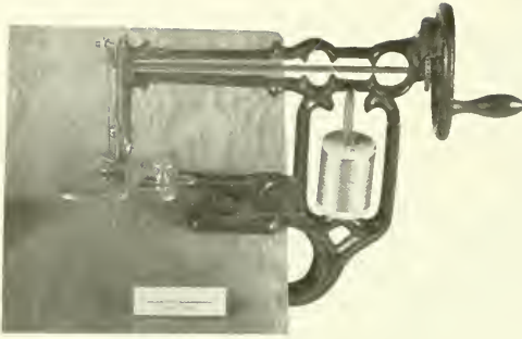
Figure 93.—HANCOCK SEWING MACHINE, 1867. One of the many inventors who turned his talents to inventing and producing a mechanically simple and cheaper machine was Henry J. Hancock. His 1867 machine is only about six inches wide; it uses a tambour-type needle, pulling a loop of thread from below the stitching surface. (Smithsonian photo P63197.)
