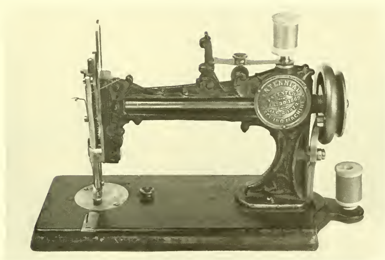
Figure 78.—CENTENNIAL SEWING MACHINE, 1876. The Centennial machine was basically a McLean and Hooper sewing machine which was renamed to take advantage of the coming Centennial celebration. It was based on the patents of J. N. McLean, March 30, 1869, and August 2, 1870, and made a two-thread chainstitch. Only about five hundred Centennial machines were manufactured in 1873, but by 1876 over three thousand had been constructed. The machines were advertised on white circulars which were printed in red and blue, and engraved with two women sewing, one by hand, labeled "Sewing in 1776," and one at a Centennial sewing machine, labeled "Sewing in 1876." There is no record that the machines were made after 1876. (Smithsonian photo 48216-T.)
