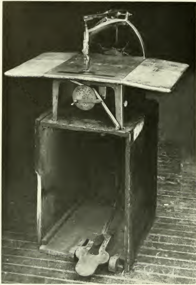
Figure 70.—AMERICAN MAGNETIC SEWING MACHINE, 1854. Machines of this type were manufactured for only two years under the patent of Thomas C. Thompson, March 29, 1853, and later under the patents of Samuel J. Parker, April 11, 1854, and Simon Coon, May 9, 1854. On September 30, 1853, Elias Howe listed receipts of $1000 from the American Magnetic Sewing Machine Co. for patent infringement. The machines manufactured after that date carry the Howe name and 1846 patent date to show
