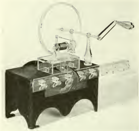
Figure 17.—MOREY AND JOHNSON sewing machine, 1849. Below: The machine is marked with the name of its maker, Safford & Williams. The number 49 is a serial number. Missing parts have been replaced with plastic. (Smithsonian photo 48400; brass plate: 48400-H.)
