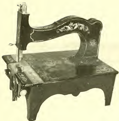
Figure 81.—EUREKA SEWING MACHINE, 1859. An example of the many short-lived types of which no written record can be found, this particular machine was used as a patent model for certain minor improvements in 1859. It has the name "Eureka" painted on the top and the following inscription incised on the baster plate: "Eureka Shuttle S. M. Co. 469 Broadway, N.Y." Although it is a shuttle machine, it carries no patent dates and was not included in the Howe royalty records. Neither is it listed in the obsolescence list published in 1881. The company probably could not pay its royalty fees and was forced out of business almost immediately. If this machine had not been used as a patent model, no record of the company's existence might remain. It should be noted that as in most shuttle machines the head was meant to be set into a treadle-powered table. Since most tables are very similar, they are not required for identification. (Smithsonian photo 48328-C.)
