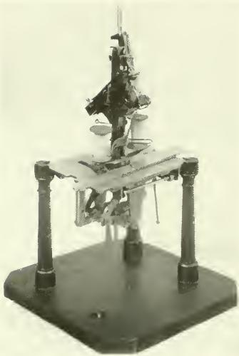
Figure 10.—MADERSPERGER'S 1839 sewing machine. Madersperger's machine consisted of two major parts: the frame, which held the material, and the stitching mechanism, called the hand. The hand shown here is an original model. (Photo courtesy of Technisches Museum für Industrie und Gewerbe, Vienna.)
