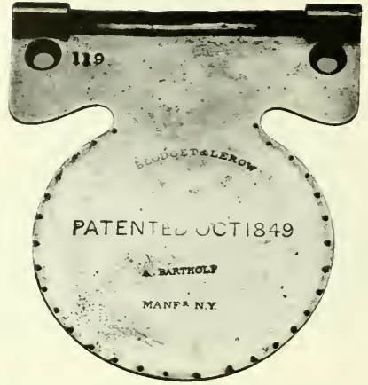
Figure 20.—BLOODLETT & LEROW SEWING MACHINE, 1850, as manufactured by A. Bartholf, New York; the serial number of the machine is 19. At right, an original brass plate from the same type of machine with needle arm and presser foot and arm, serial number 119; the plate, however, does not fit the machine correctly. (Smithsonian photo 48440-D; brass plate: 48440-K.)
