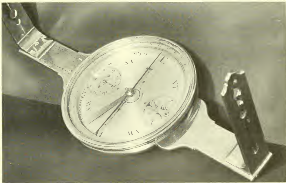
Figure 28.—Brass surveying compass made by Goldsmith Chandlee for Laurence Augustine Washington in about 1795. In the library at Mount Vernon. Photo courtesy the Mount Vernon Ladies Association of the Union.
