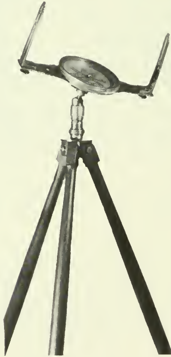
Figure 4.—Surveying compass marked “Potts and Rittenhouse.” Believed to be the work of David Rittenhouse in partnership with Thomas Potts. Photo courtesy the American Philosophical Society.
