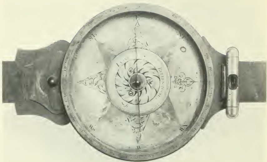
Figure 81.—Brass surveying compass marked “Rittenhouse & Evans,” about 1780. Over-all length, 13\frac{3}{4} in.; diameter of dial, 5\frac{1}{4} in. This instrument, made about 1780, was owned and used by John Johnson in 1818 for surveying the boundaries between Canada and Maine. USNM 309543.
