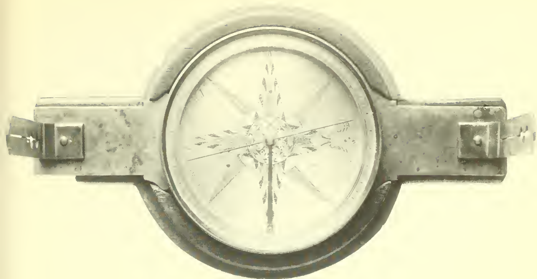
Figure 79.—Surveying compass made by David Rittenhouse for Gen. George Washington, inscribed “Rittenhouse, Philadelphia.” This instrument was used by Washington in making a complete survey of his estate at Mount Vernon, 1796–1799. The survey was assisted by Capt. Samuel Duval, surveyor of Frederick County, Maryland. Washington gave the instrument to Captain Duval, from whom it descended to the Hon. Anthony Kimmel, who donated it to the U.S. National Museum. USNM 92538.
