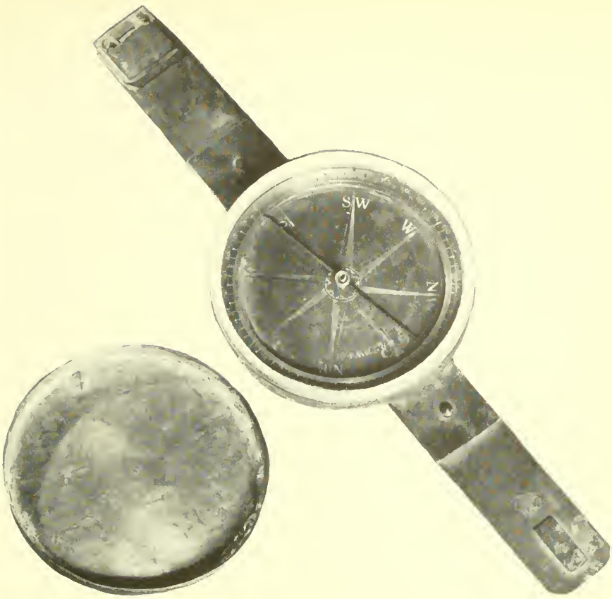
Figure 17.—Brass surveying compass made by Stephen Greenleaf (fl. 1745) of Boston. Photo courtesy New Hampshire Historical Society, Concord.
