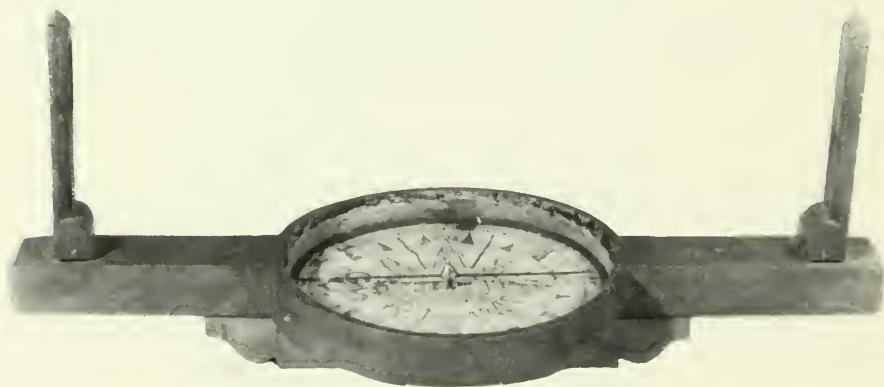
Figure 61.—Wooden surveying compass made by Benjamin Warren (c.1740–c.1800) of Plymouth, Massachusetts, and detail of the compass card. The compass, made of cherry wood, is 12 in. long and has a diameter of 6 in. In Streeter Collection of Weights and Measures, Yale University.
