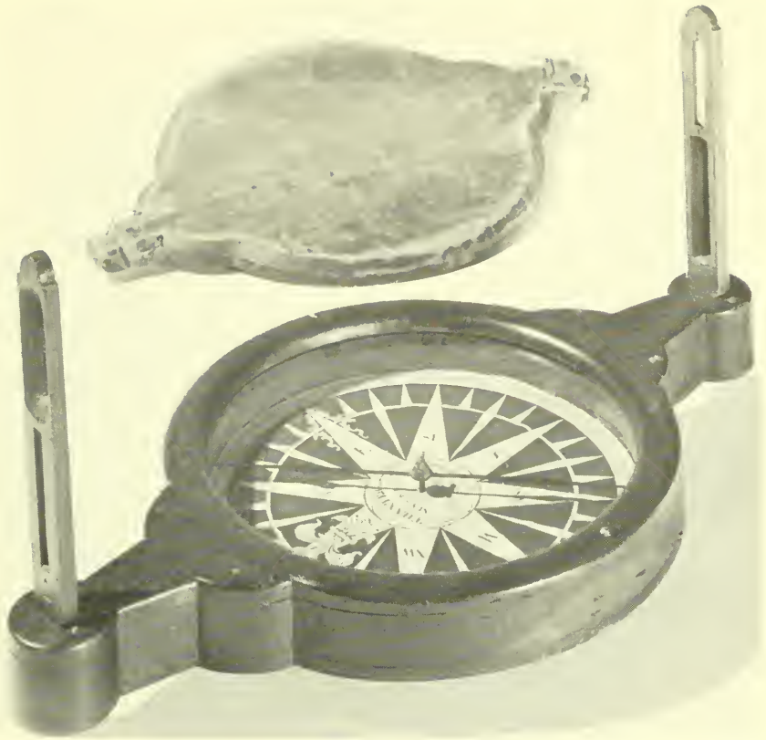
Figure 52.—Mahogany surveying compass made by Samuel Thaxter of Boston. Length, 13 in.; diameter, 7\frac{1}{2} in. Wooden frame slides off to permit removal of glass and adjustment of needle. Sighting bars are of boxwood. In collection of the writer.
