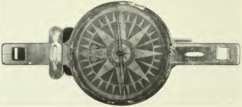
Figure 67.—Wooden surveying compass made by Thomas Salter Bowles of Portsmouth, New Hampshire. With spirit level. Made of birch, the compass is 13 in. long and has a diameter of 6 in. In the Streeter Collection of Weights and Measures, Yale University.
