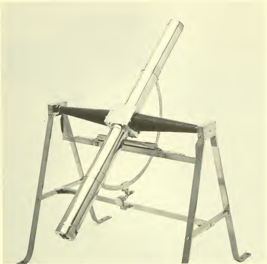
Figure 3.—Transit telescope made by David Rittenhouse and used by him for the observation of the transit of Venus in 1769. Brass, 33\frac{1}{2} -in. tube on a 25-in. axis, with an aperture of 1\frac{3}{4} in. and a focal length of 32 in. Photo courtesy the American Philosophical Society.
