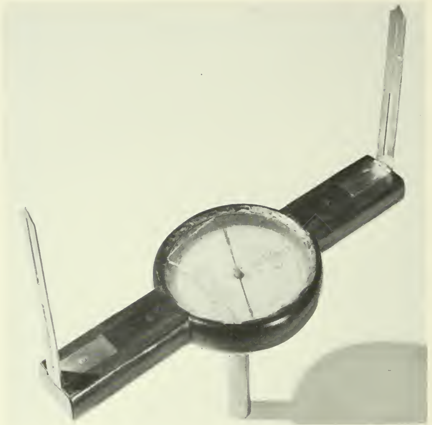
Figure 66.—Views of wooden surveying compass made by Gurdon Huntington, clockmaker in Walpole, New Hampshire, between 1789–1804. Made of cherry with folding brass sighting bars, the instrument is 14 in. long and 5\frac{1}{2} in. wide. In collection of the writer.
