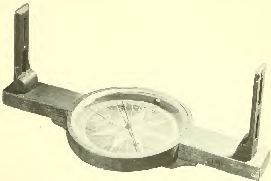
Figure 43.—Wooden surveying compass, made and sold by Thomas Greenough. The instrument is made of gumwood and has a paper compass card; it is 13\frac{1}{4} in. long and has a diameter of 5\frac{1}{4} in. In collection of Franklin Institute, Philadelphia.
