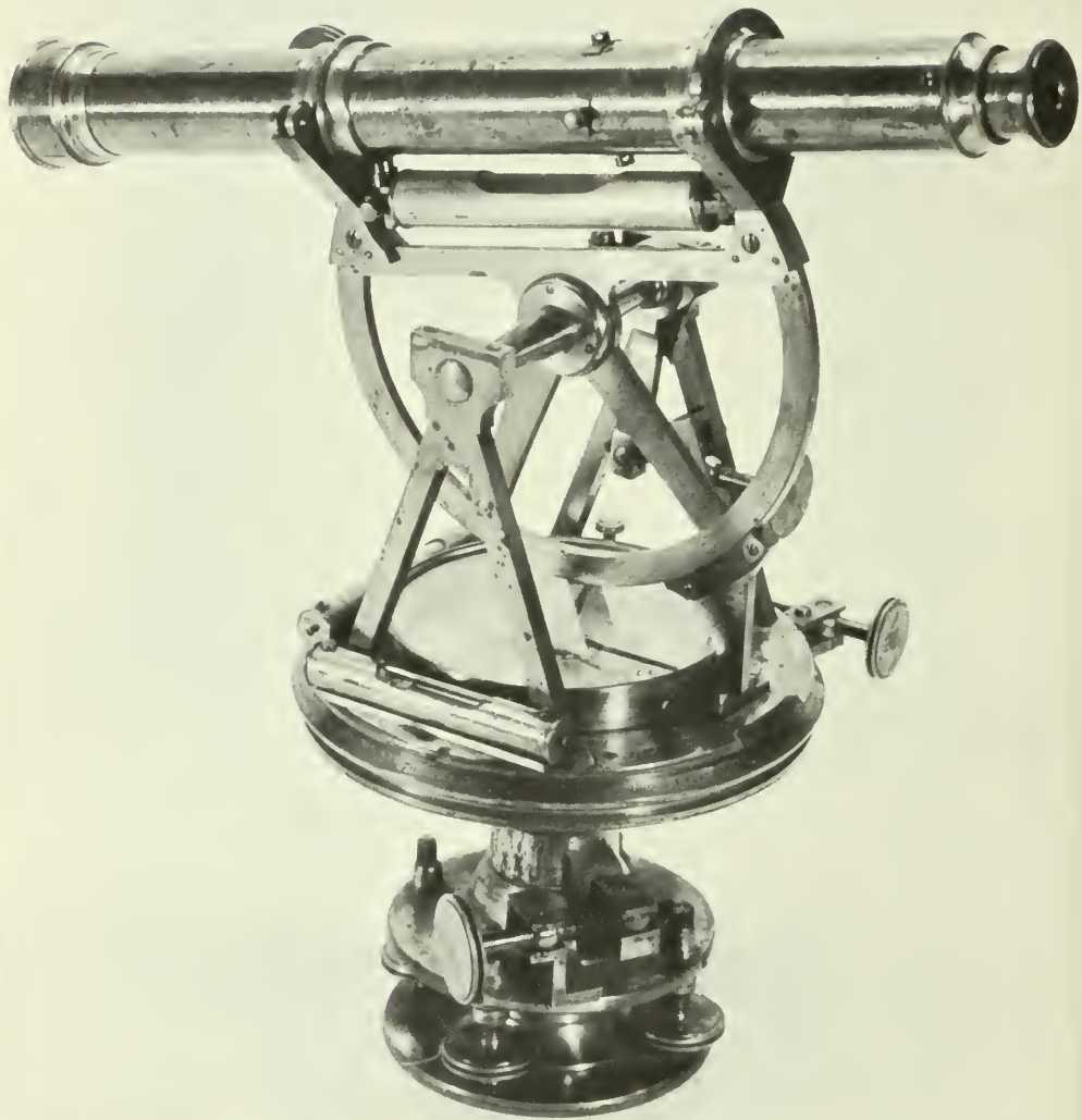
Figure 25.—Surveying theodolite made by Augustus Platt (1793–1886) of Columbus, Ohio, in the early 19th century. Photo courtesy Ohio State Museum.
