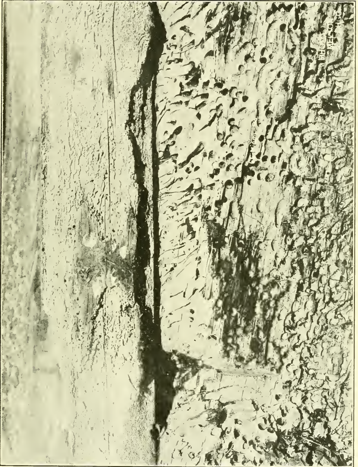
RAVAGES BY GOULD SHIPWORM AT MIAMI, FLORIDA.
