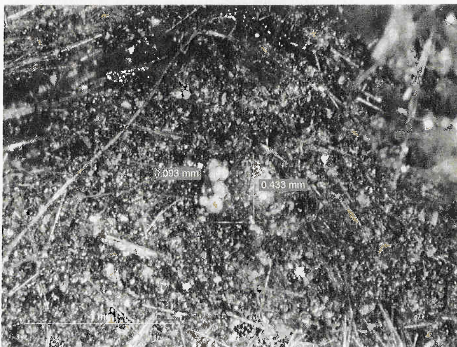
Fig. 3b The fiberglass matrix impregnated with nylon-phenolic resin cloth; surface analysis microscope, Olympus LEXT OLS4000, IEDF image.
