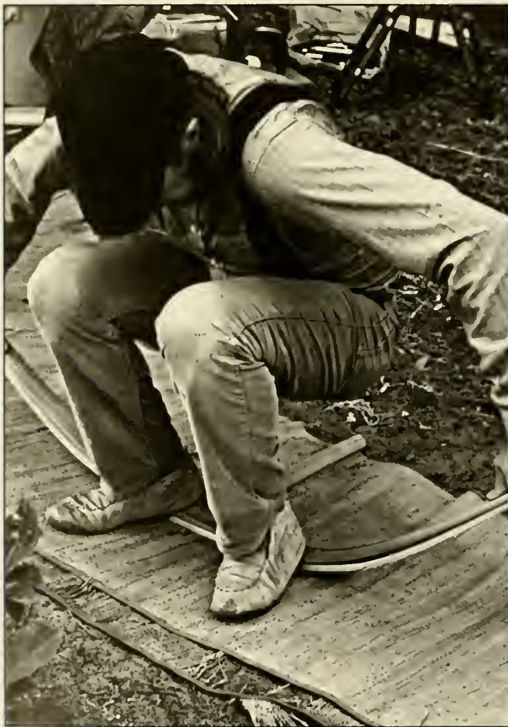
Fig. 4. Earl Nyholm bends canoe ribs, using two at a time to guard against breakage. Photo by Janet Cardle
