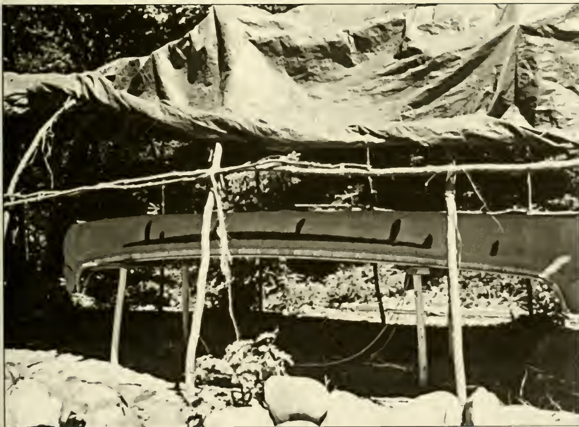
Fig. 6. The 14-foot canoe, inverted for “gumming” (“pitching”) all cut and sewn areas on the bark, is ready for launching.
