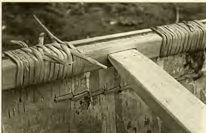
Fig. 2. This detail of the gunwale assembly shows the tapered end of the thwart inserted into the mortise of the inwale, split jackpine roots for lashing, and double-stitch sewing.
