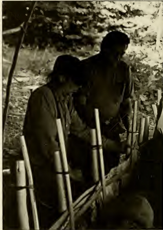
Fig. 1. Earl Nyholm and Charlie Ashmun tie inner stakes to exterior canoe form-stakes. Note the boulders weighting down the canoe form; also, that the white outer bark of the tree becomes the inside of the canoe.
