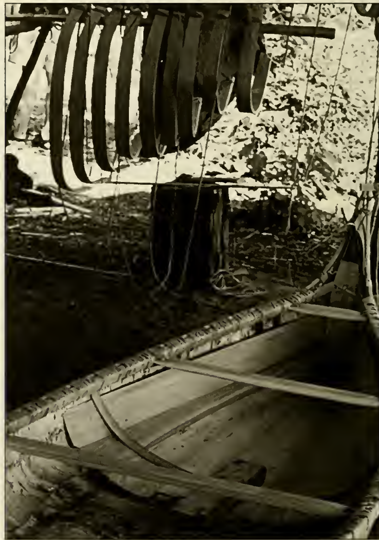
Fig. 5. View of the interior of the canoe with some of the thin cedar planking in place. Note the hanging bent and dried ribs which will be reinserted once the flooring is completely set in place. Photo by Janet Cardle
