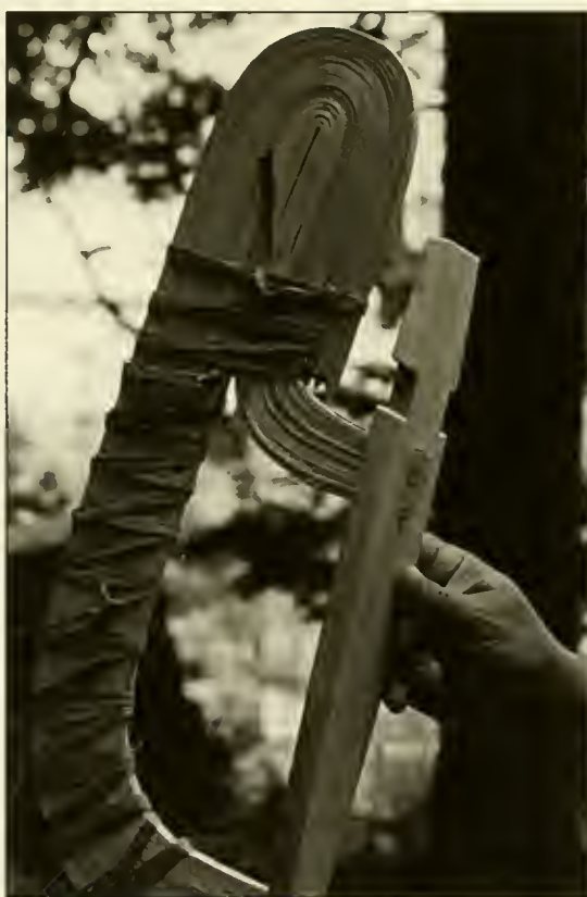
Fig. 3. Canoe-prow assembly with "man-board" — so called because it resembles a human form. A single piece of cedar is used which is split into more than 30 laminations to effect the bends in its form. These are held in place using wigoob (the inner bark of the basswood tree) and threaded through and inserted over the man-board. Photo by Janet Cardle
