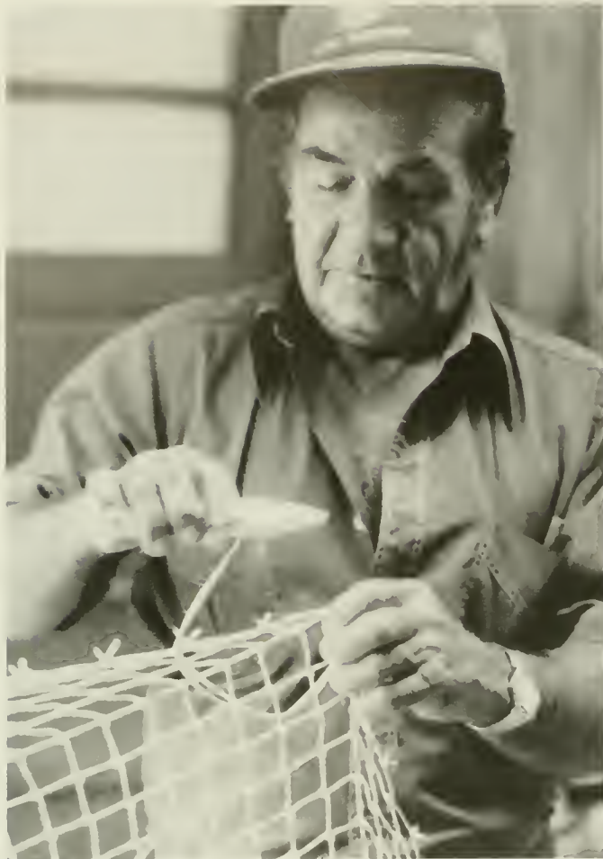
Otis Smith sewing the selvaige along the tapered edge of a trap-net pot piece. Photo by Janet Gilmore
