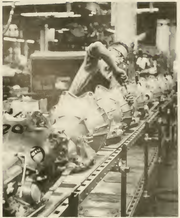
Pontiac Tech IV “double e” assembly line allows an engine to stop at each work station along the line, enabling the operator to control the work unit. Photo courtesy Motor Vehicle Manufacturers Association Archive
