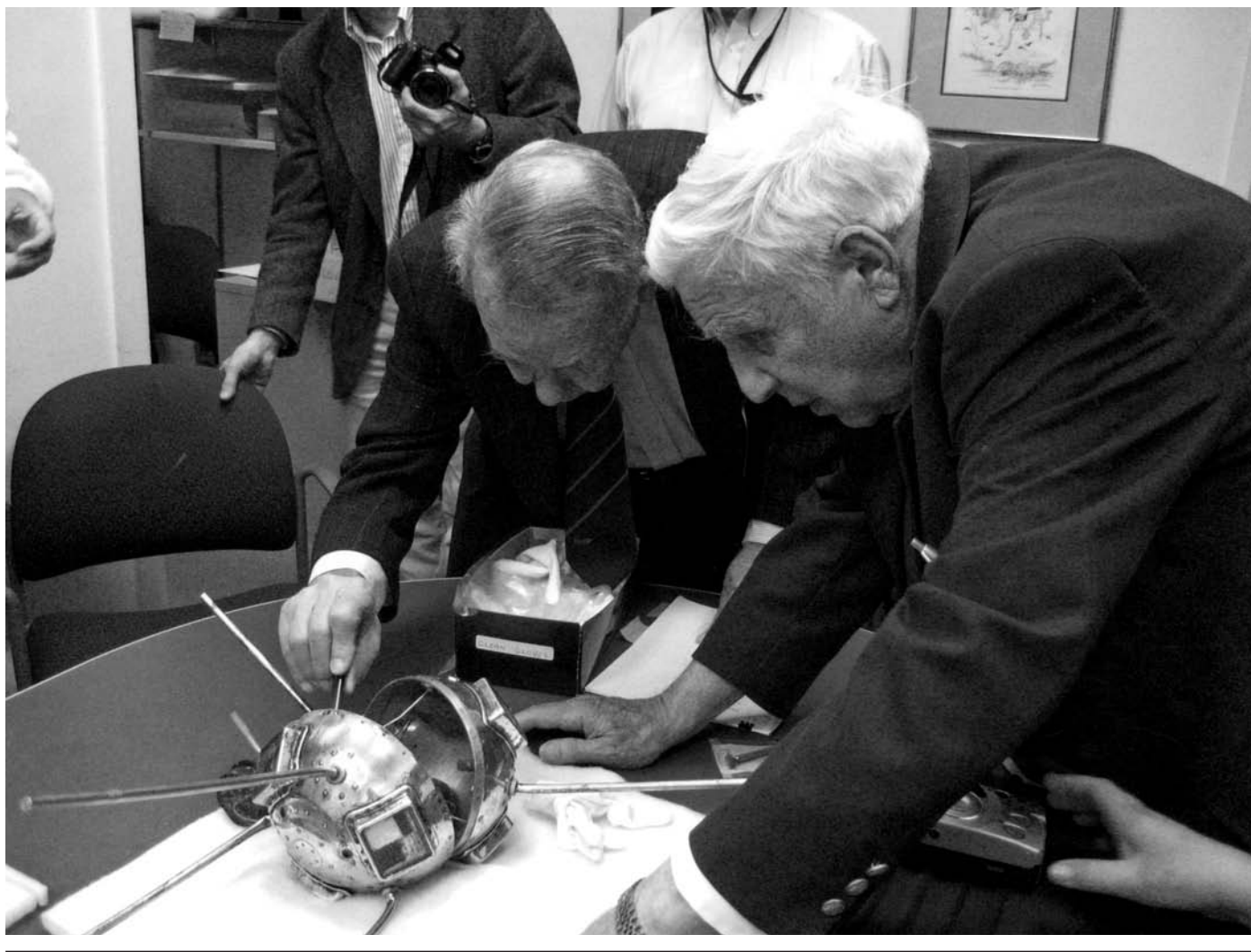
FIGURE 3. Examination of the original TV-3 satellite in March 2008, by members of the Naval Research Lab team who designed and built it, on the eve of the fiftieth anniversary of the first successful Vanguard flight. The object was opened to allow inspection for identification of components, search for undocumented experiments, and to assess its state of preservation. Martin Votaw, left, Roger Easton, right. (Photograph courtesy Judith Pargamin)
