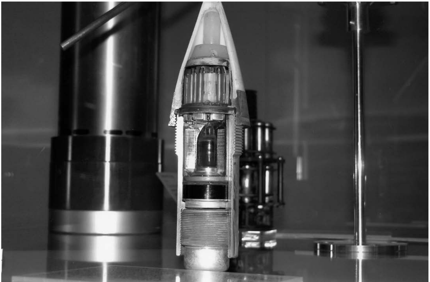
FIGURE 9. World War II-era Mark 58 radio proximity fuze for anti-aircraft artillery fire control designed by the Applied Physics Laboratory group that included Van Allen. (NASM photograph)
