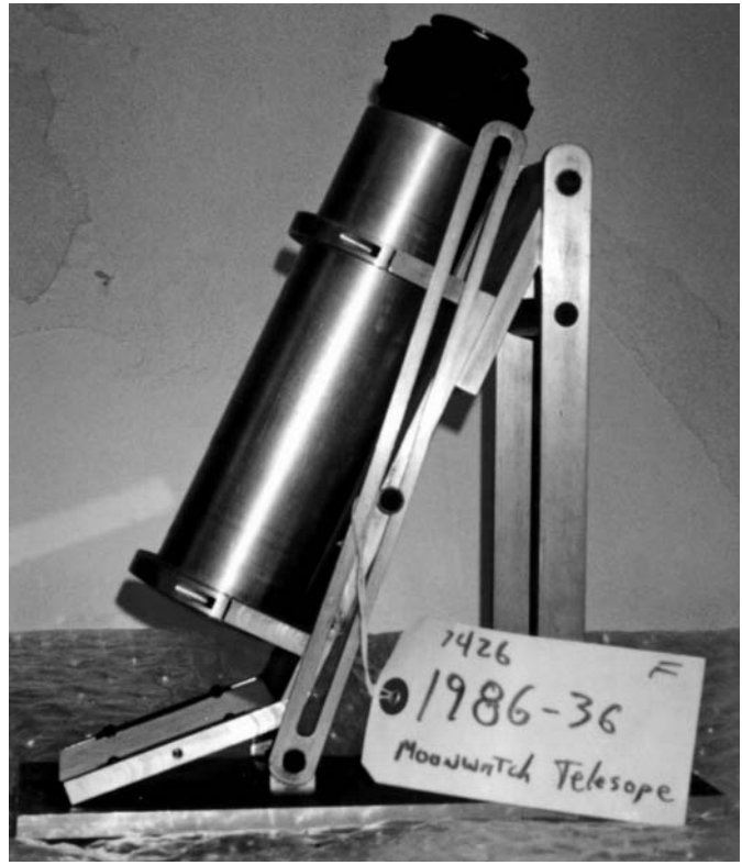
FIGURE 1. Project Moonwatch telescope (A19860036000), preserved and on display at the NASM's Hazy Center. Amateurs and commercial organizations alike built thousands of instruments of this type; they exist in many forms. The Smithsonian Astrophysical Observatory created and coordinated the Moonwatch program to produce preliminary orbital elements of the first satellites. (NASM photograph)
