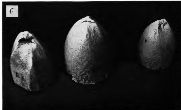
c , Iodine salt cakes (initially right circular cylinders) after erosion at 4.8 knots for (left to right) 18 minutes, intermittent; 16 minutes, steady; and 21 minutes, intermittent.
