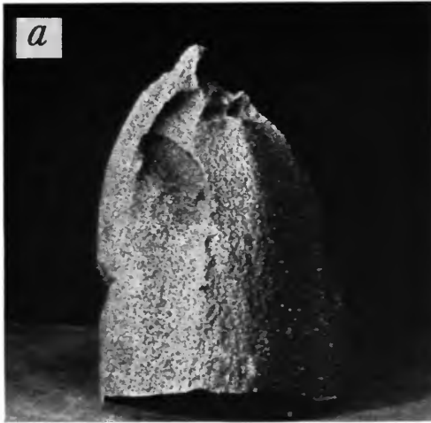
a , Blue salt cake (initially a right circular cylinder) after erosion at 4.8 knots for 16 minutes with attitude not adjusted.
