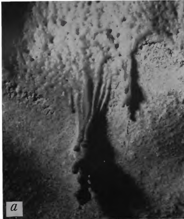
a , Enlargement of region "b" of text figure 1, showing reversed flow just upstream of point of impingement of rocket blast. Flow direction is marked by a streamer of glass terminating in a knob formed by surface tension.
