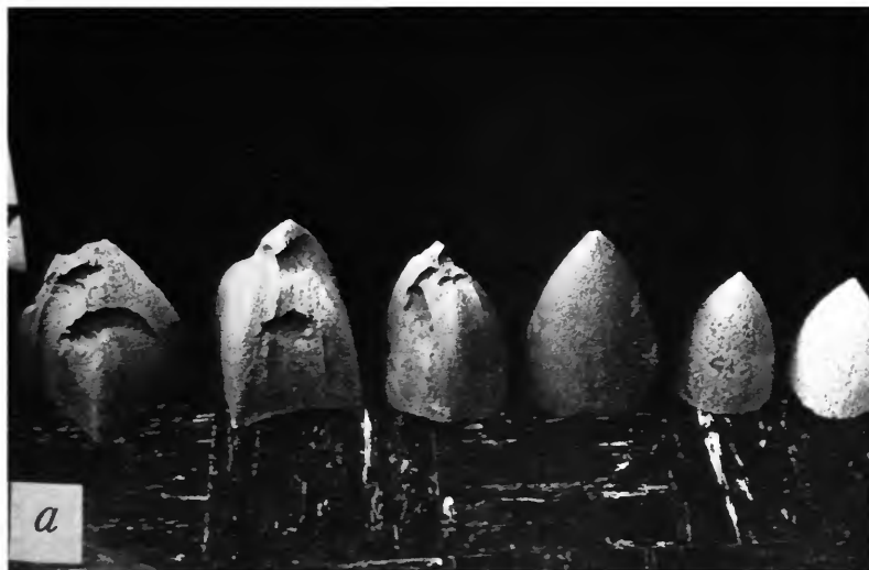
a , Blue salt cakes after erosion at different lengths of time and speeds. Only the three unpitted shapes on the right were both symmetrical initially and adjusted as to attitude; of these, the cake at the far right was a right circular cylinder and the other two were ogives. The difference in color of the cake furthest right suggests variation in composition.
