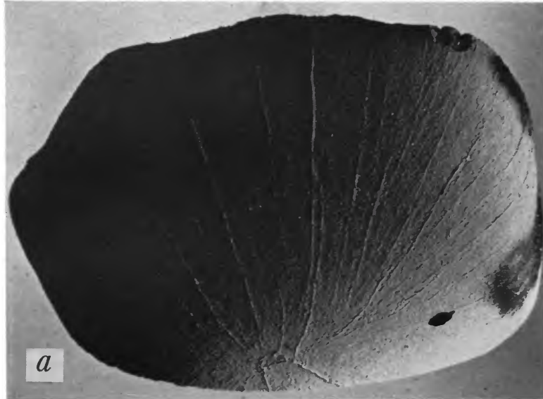
a , Leading face of the Lafayette stone, with stagnation region near the bottom. The airflow, smooth and producing no pitting, is clearly marked by flow lines. Flow left the stone where the top edge of the face is marked by a skirt of slag.
