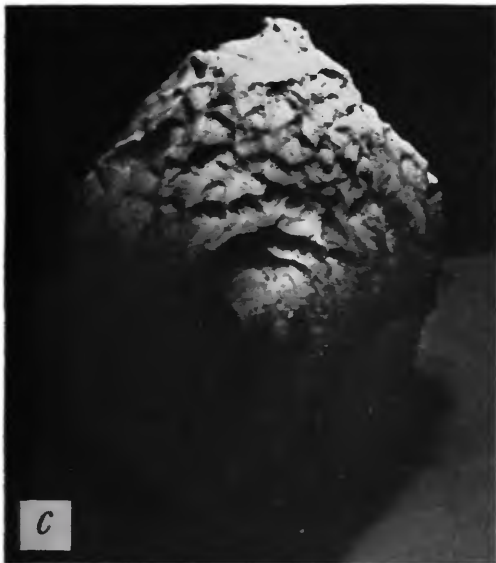
c , Iodine salt block after erosion for 16 minutes at 3.1 knots. Pitting is extensive on the leading face, a characteristic of low speed erosion on bluff objects.
