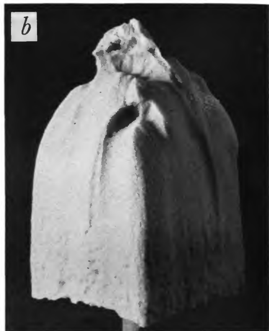
b , Iodine salt block after erosion for 8 minutes at 4.1 knots. Note orderly pit system on the leading end and the small pits near the base, far from the tip.
