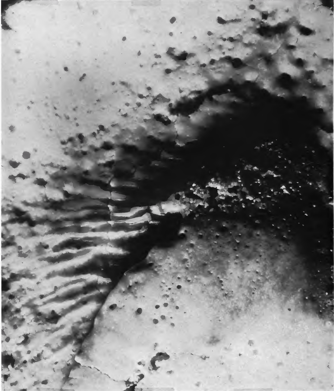
Enlargement of a crest region in the eroded ceramic plate pictured in plates 1 and 2. The main flow is upward. Due to a vortex in the boundary layer the flow in the lee of the crest is roughly at right angles to the main flow, as indicated by the glass rivulets terminating in a knob.
