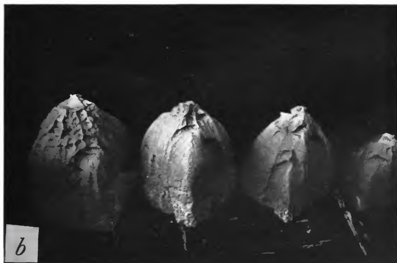
b , Iodine salt cakes (initially rectangular blocks) after 16 minutes at (left to right) 3.1, 4.1, 4.8, and 5.5 knots.
