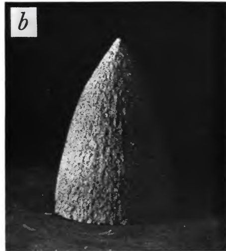
b , Blue salt cake (initially a right circular cylinder) after erosion at 4.8 knots for 21 minutes with attitude adjusted.
