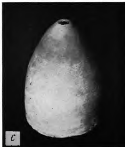
c , Ogive machined from salt block ( b ).
