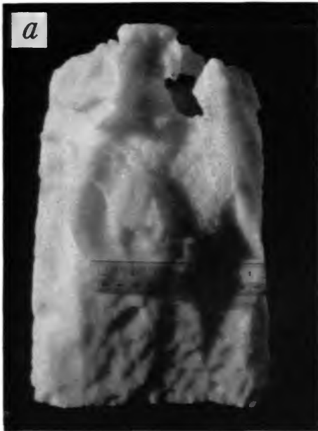
a , White salt block after erosion for 8 minutes at 4.1 knots, showing irregular erosion and deep pitting. Eroded shapes are so intricate that interpretation of water flow is difficult.
