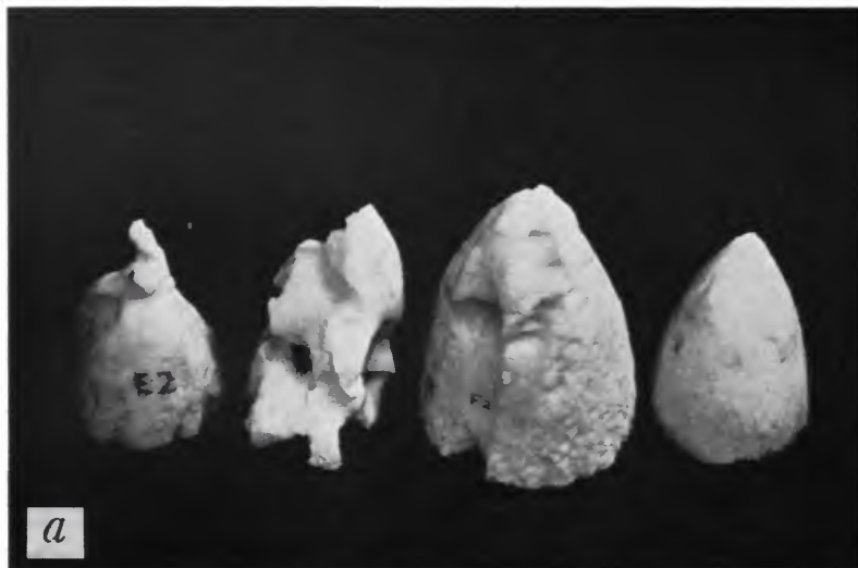
a , White salt cakes (initially symmetrical) after erosion at 4.8 knots for (left to right) 14, 14, 8, and 12 minutes. The first block on the left was the only one not adjusted as to attitude. The first two cakes on the left were right circular cylinders; the other two were ogives.
