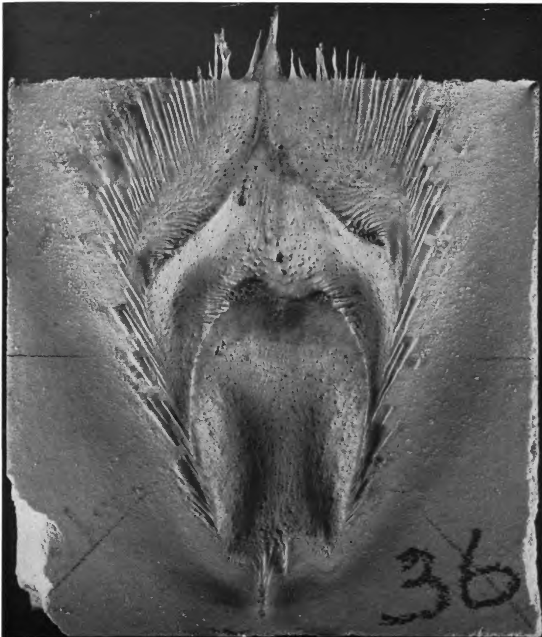
Erosion pattern carved in a ceramic plate by a rocket blast, with evidence of reversed flow at the bottom. As the blast "bounced" along the surface, it created vortices in the boundary layer between the plate and the blast.
