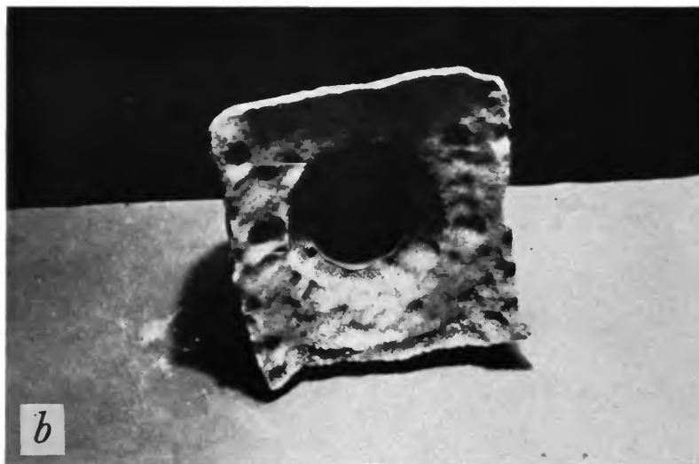
b , Base of an iodine salt cake after erosion at 5.5 knots for 16 minutes, typical of all base areas on eroded bodies. Note the broad and shallow depressions and striking resemblance to meteorite trailing faces.
