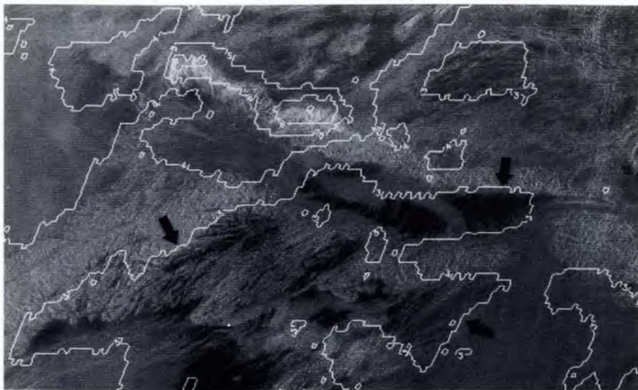
FIG. 16. Magellan radar image of plains and tessera units with contours of dielectric constant overlaid (30.5–34.0°S, 39.0–45.5°E). Contour values plotted for \epsilon values of 2, 3, 4, 5, 6, 7, and 8. Note the low values of \epsilon (3.0 contour marked by black arrows) associated with the radar-dark lava flows.
