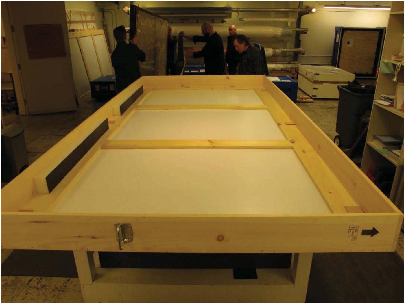
Figure 2. The travel box is made of wood. Ethafoam and Volara inserted in the bottom of the box absorb shock and vibration, and Coroplast covers the front and back of the box
