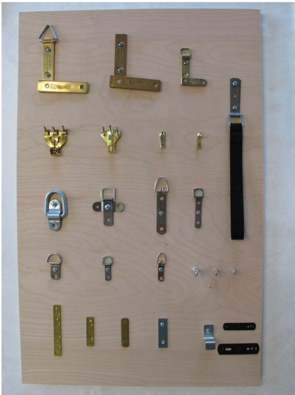
Figure 5. Sample board illustrating various types of hanging hardware. Top row from left to right on the display board are two sizes of Oz-clips with D-ring and one without D ring
