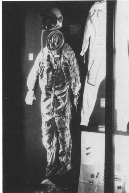
Fig. 2. A project Mercury spacesuit that has been on exhibit since 1976. The exhibit techniques that are contributing to the spacesuit's deterioration include improper support, internal fluorescent lights at close proximity to the suit and uneven lighting.
