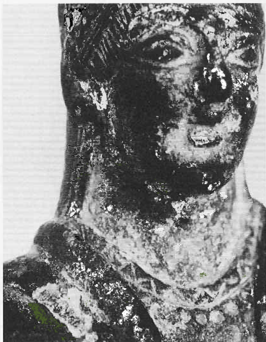
Figure 37. A copper-tin alloy object showing typical bronze disease. See color plate h.
